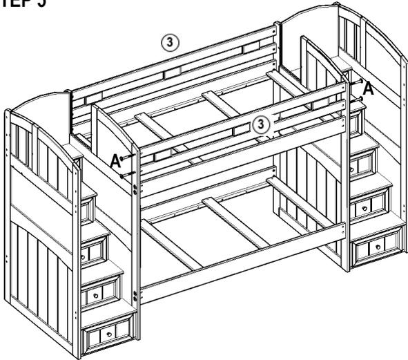
Assemble guardrails and tighten all bolts.
