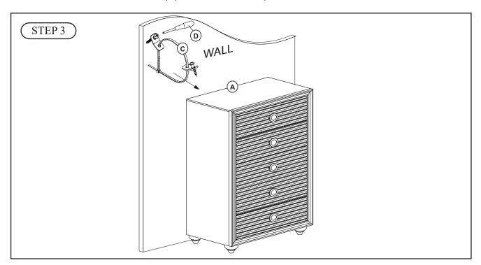
To prevent the Chest (A) from tipping, mount one side of the Tipping Restraint (C) to the backside of the Chest (A) and the other side to the wall.
