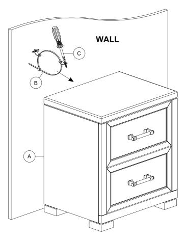
To prevent the Nightstand (A) from tipping, mount one side of the Tipping Restraint (B) to the backside of the Nightstand (A) and the other side to the wall.
