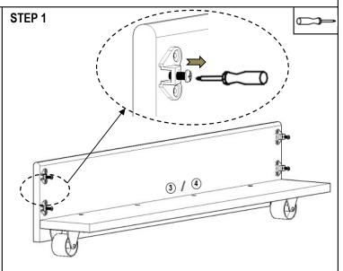
Remove the four screws in both side panels and save for re-attach.
