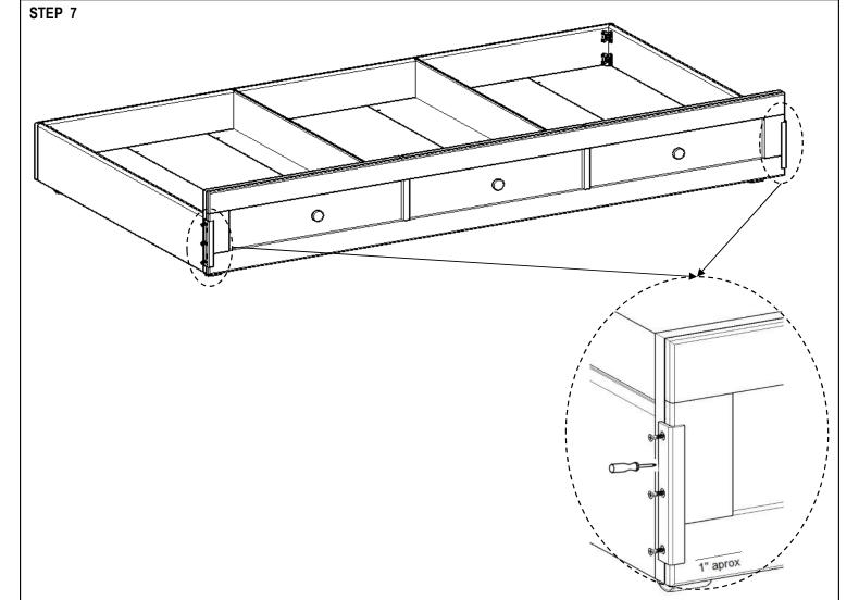
Install plastic plates, one in each front side as shown, fasten with three screws.
