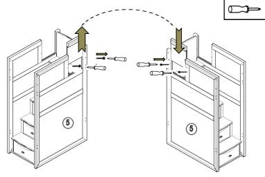
For stairs on the left, first remove the screws, then remove the panel and install it on the other side and secure with the screws.
