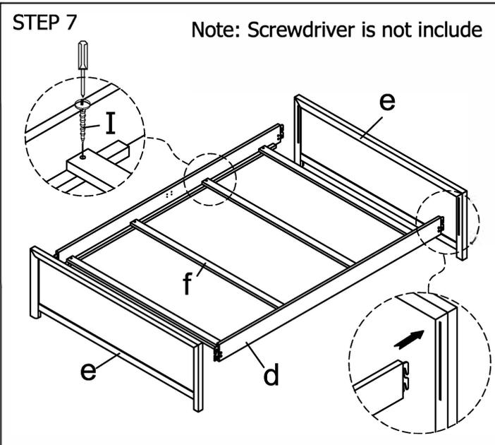
Attach Side rails to two Twin or Full Footboard. Then screw all slats to Side rails.
