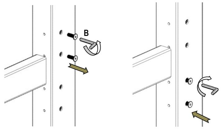
Remove bolts from top setting then install in the lower setting, do not tighten, allow 1/4" space between post and bolt head, repeat for all posts.
