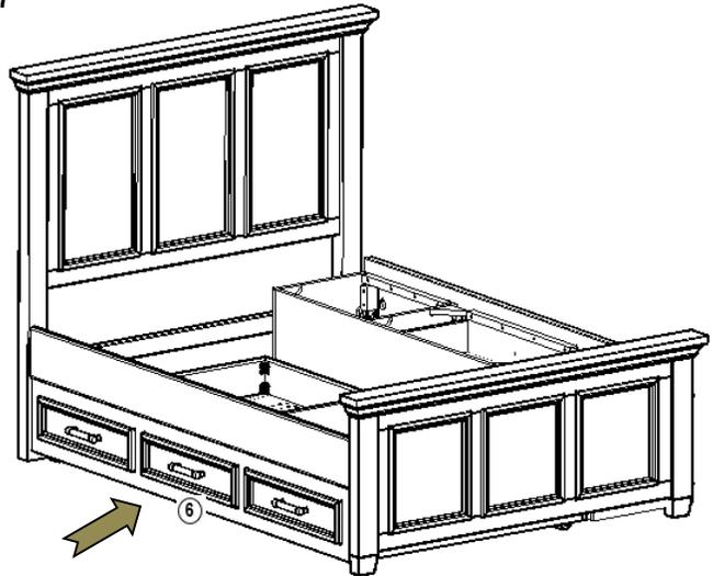
Install slats, one on each space between the small blocks, then fasten with 1 1/4" screws.
