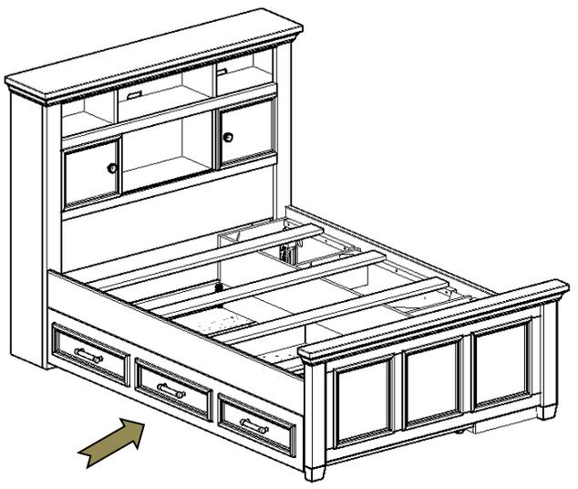
For optional Trundle bed follow assembly instructions inside tighten, allow 1/4" space between post and bolt head, repeat for all posts.
