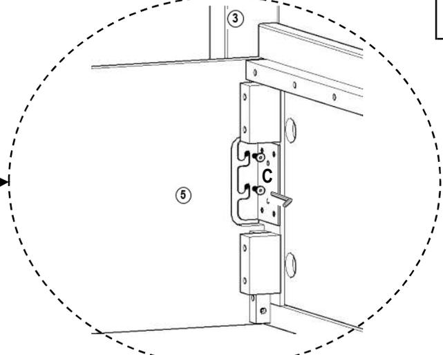
Assemble pedestal first aligning the pedestal bracket with holes in the bottom set of holes of the headboard and footboard then fasten using the bolts previously removed **MAKE SURE ALL BOLTS ARE TIGHTENED COMPLETELY.**
