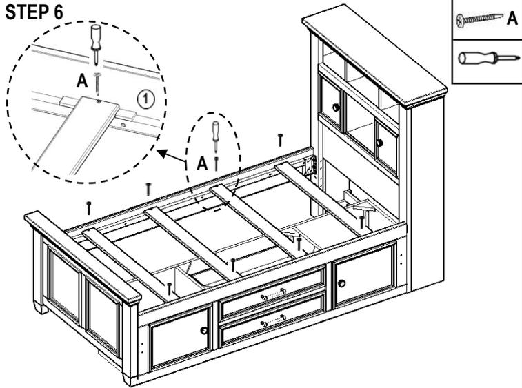
Install slats, one on each space between the small blocks, then fasten with 1 1/4" screws.
