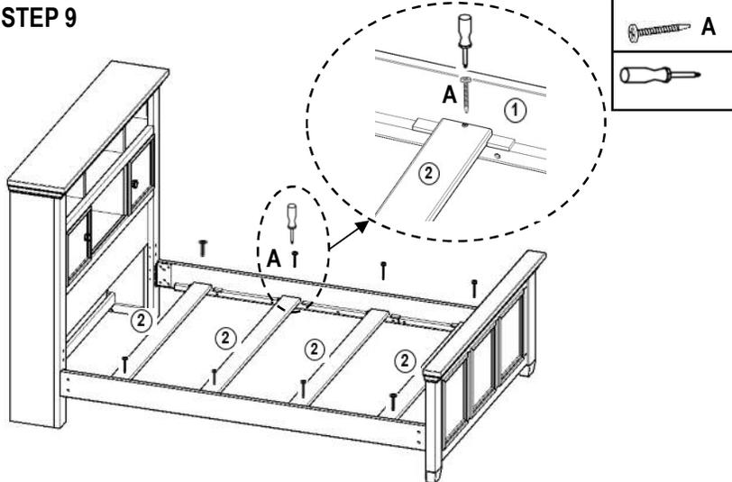
Install slats, one on each space between the small blocks, then fasten with 1 1/4" screws.
