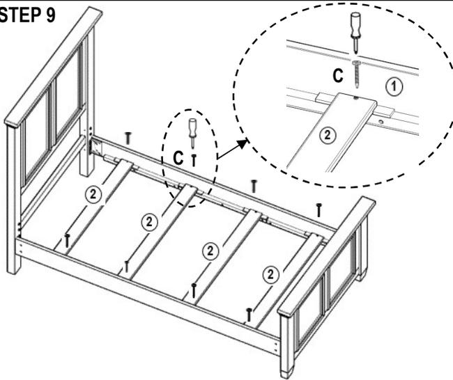
Install slats, one on each space between the small blocks, then fasten with 1 1/4" screws.
