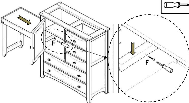
For desk on the left, open the door and secure it with one 3/4" screw (from desk box hardware pack).
