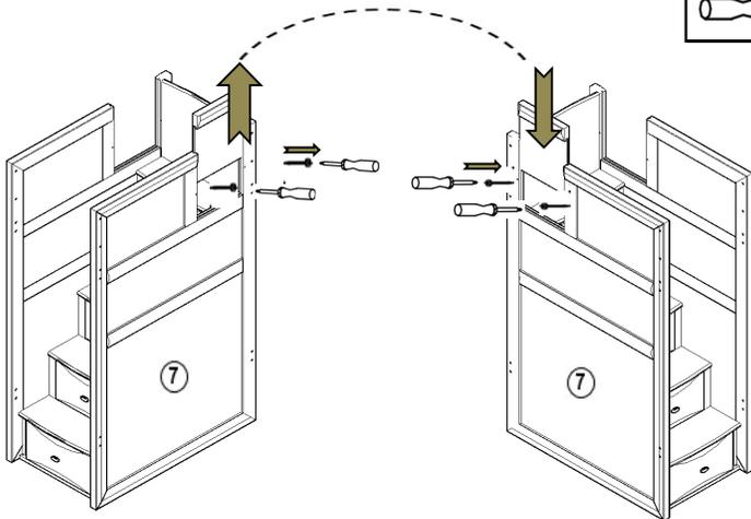
For stairs on the left, first remove the screws, then remove the panel and install it on the other side and secure with the screws.
