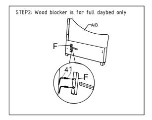
For full size Headboard(A) & Footboard(B), attach the Wood blocker (F) with bolts (1), tighten the bolt (1) with Allen key (4) as shown.
