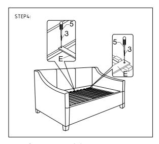
Place Straight slats(E) on the support rails as STEP4 shows.
