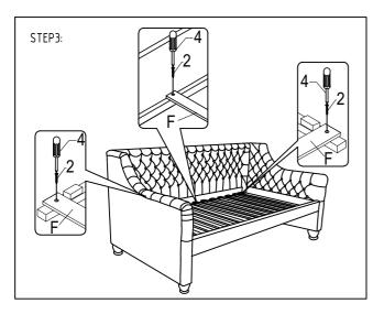
Place Straight slats on the support rails as STEP3 shows. Then secure slats by screw at spot F as STEP3 shows.
