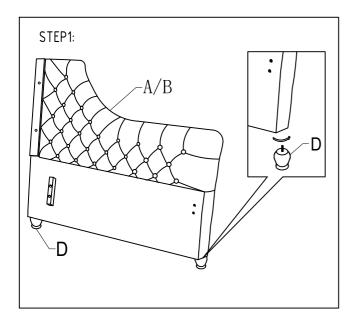
Attach the LEGS(D) on L side panel(A) and R side panel(B)
