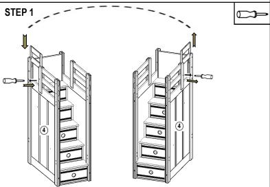
For stairs on the left, first remove the screw, then remove the panel and install it on the other side and secure with the screw.
