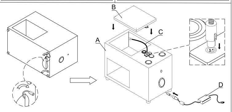
Remove the Led Light and the Charger Cord from Box. Then connect them into position.
