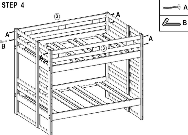
Assemble guardrails and tighten all bolts.
