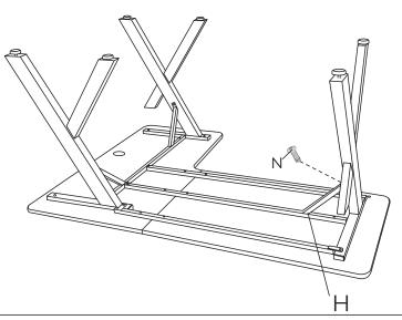
Attach the brackets to the Small Desk Top by using Allen Bolt and Allen Wrench.
