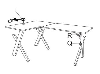
Attach the Small Desk Top to the table top by using Allen Bolt and Allen Wrench. Please fully tighten the bolts.
