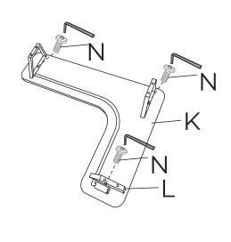
Please Push the wireless charger into the table top. Attach the hooks to the table top by using hook screw.
