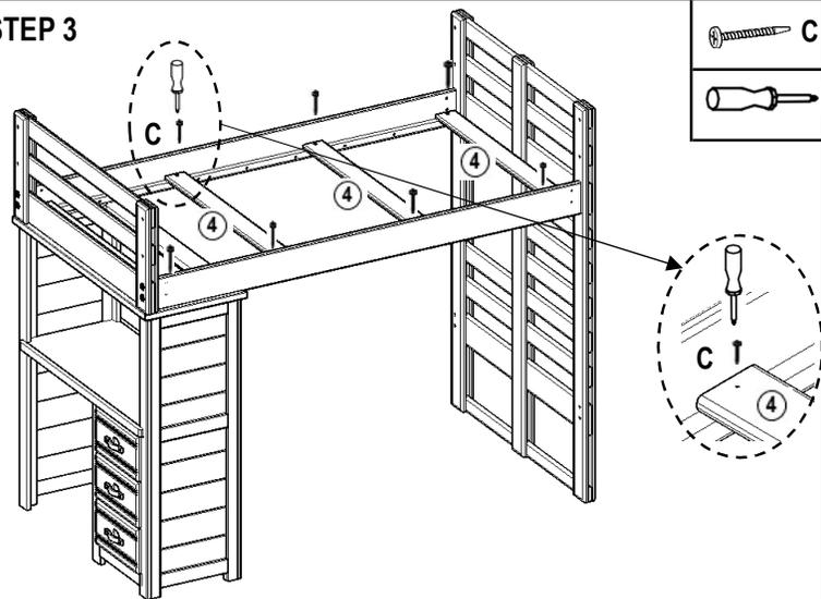
Install slats, one on each end, two equally spaced in the middle, then fasten with 1 1/4" screws.
