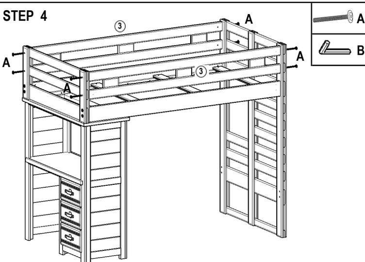
Assemble guardrails and tighten all bolts.
