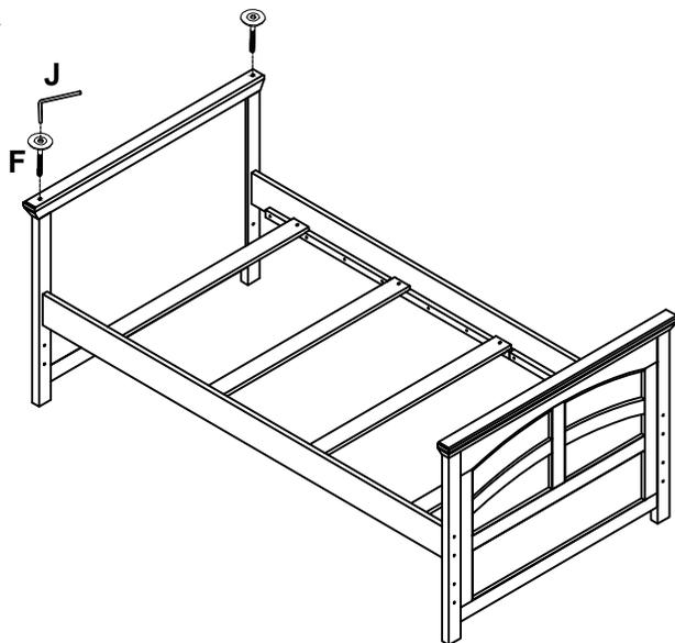
Attach bolts in pre-drilled holes on the top of lower bed end.
