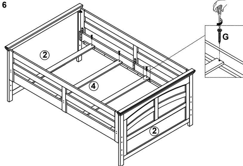
Assemble slats to side rail cleats for upper bed ends.
