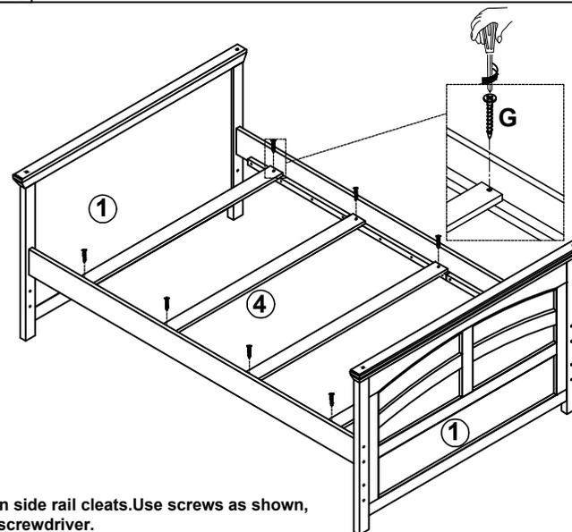
Place slats on side rail cleats. Use screws as shown, tighten with screwdriver.
