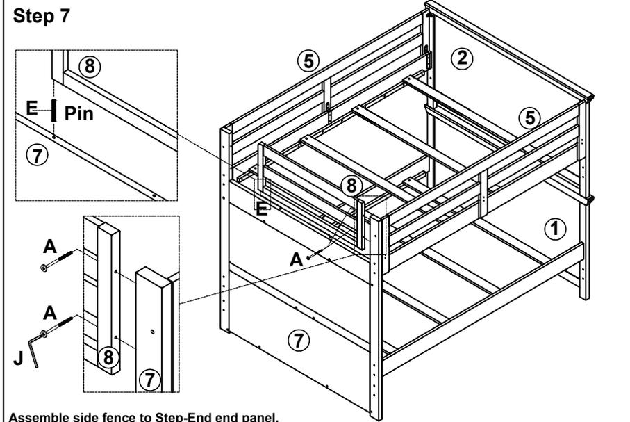
Assemble side fence to Step-End end panel.
