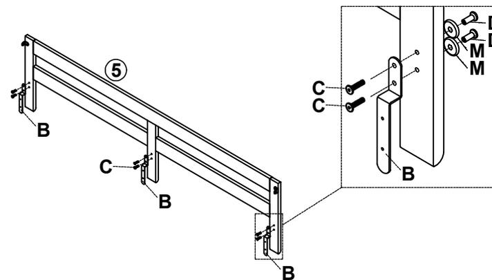
Assemble metal plates to guard rails. Complete this process for both guard rails.
