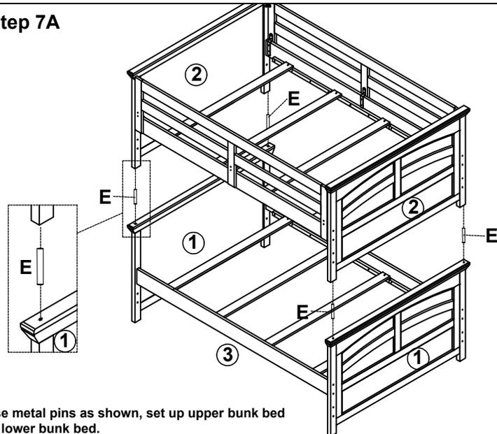
Use metal pins as shown, set up upper bunk bed to lower bunk bed.
