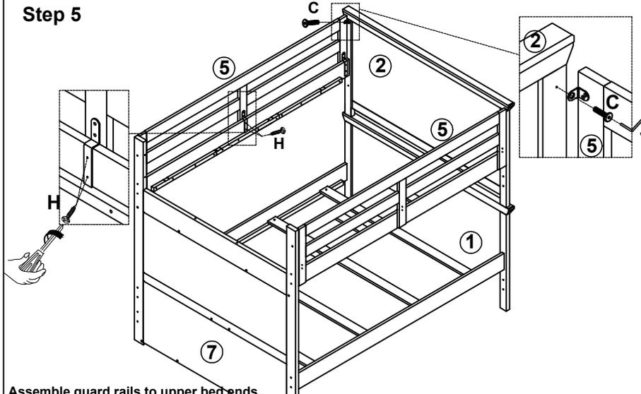
Assemble guard rails to upper bed ends.
