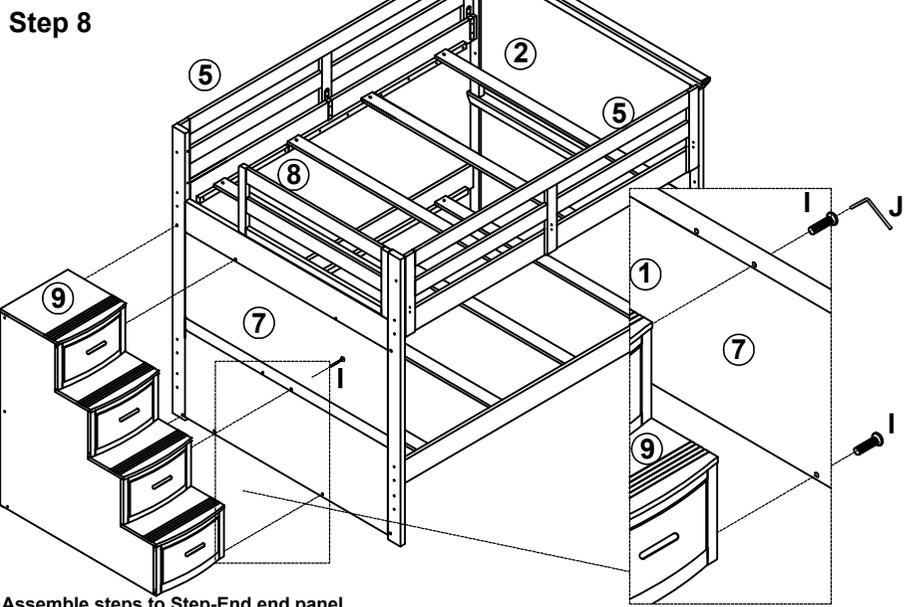
Assemble steps to Step-End end panel.
