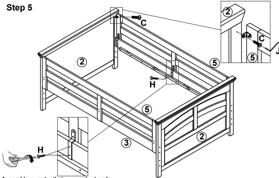
Assemble guard rails to upper bed ends.
