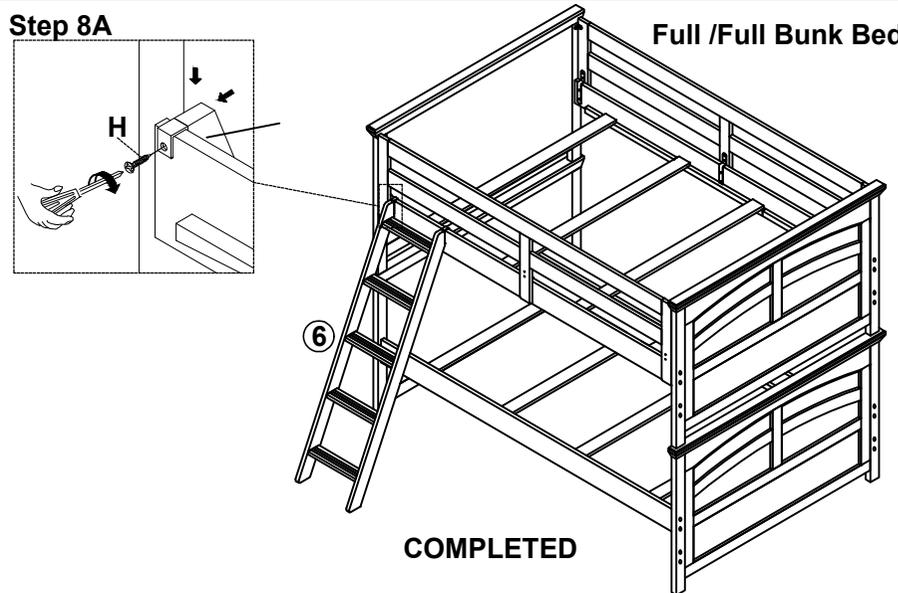
Screw ladder to upper side rail to complete assembly.
