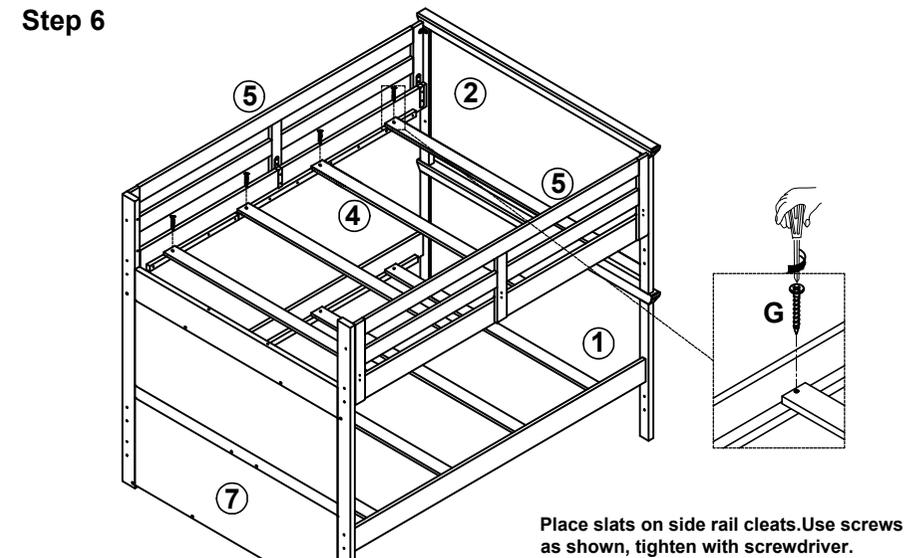
Place slats on side rail cleats. Use screws as shown, tighten with screwdriver.
