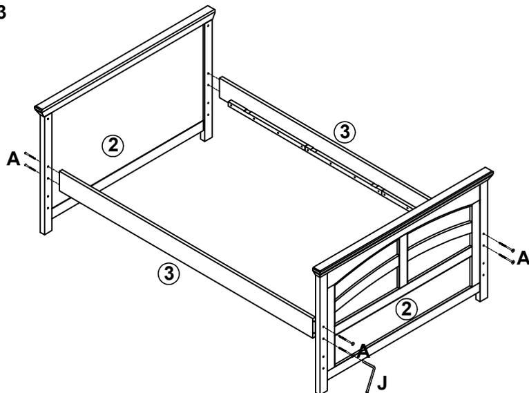
Assemble side rails to upper bed ends.
