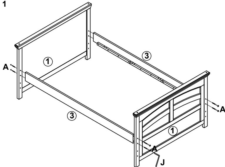
Assemble side rails to lower bed ends.
