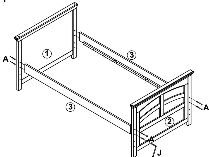
Assemble side rails to lower and upper bed ends.
