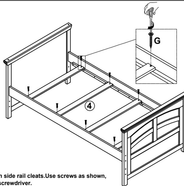
Place slats on side rail cleats. Use screws as shown, tighten with screwdriver.
