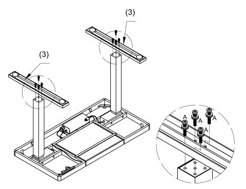
Note: Please adjust any parts out of alignment and full tighten the bolts before assemble the following steps, to prevent the looseness.
