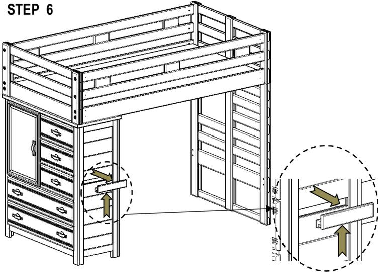
Remove center molding by lifting up then pulling out
