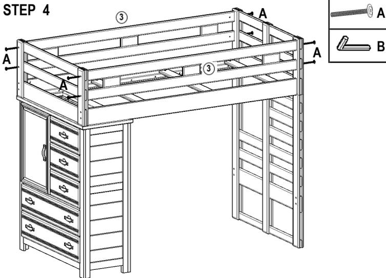
Assemble guardrails and tighten all bolts.
