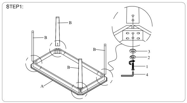
Attach table leg(B) to table top with apron (A) . Tighten by allen bolt (1), lock washer (2) and flat washer (3) with allen key (4).
