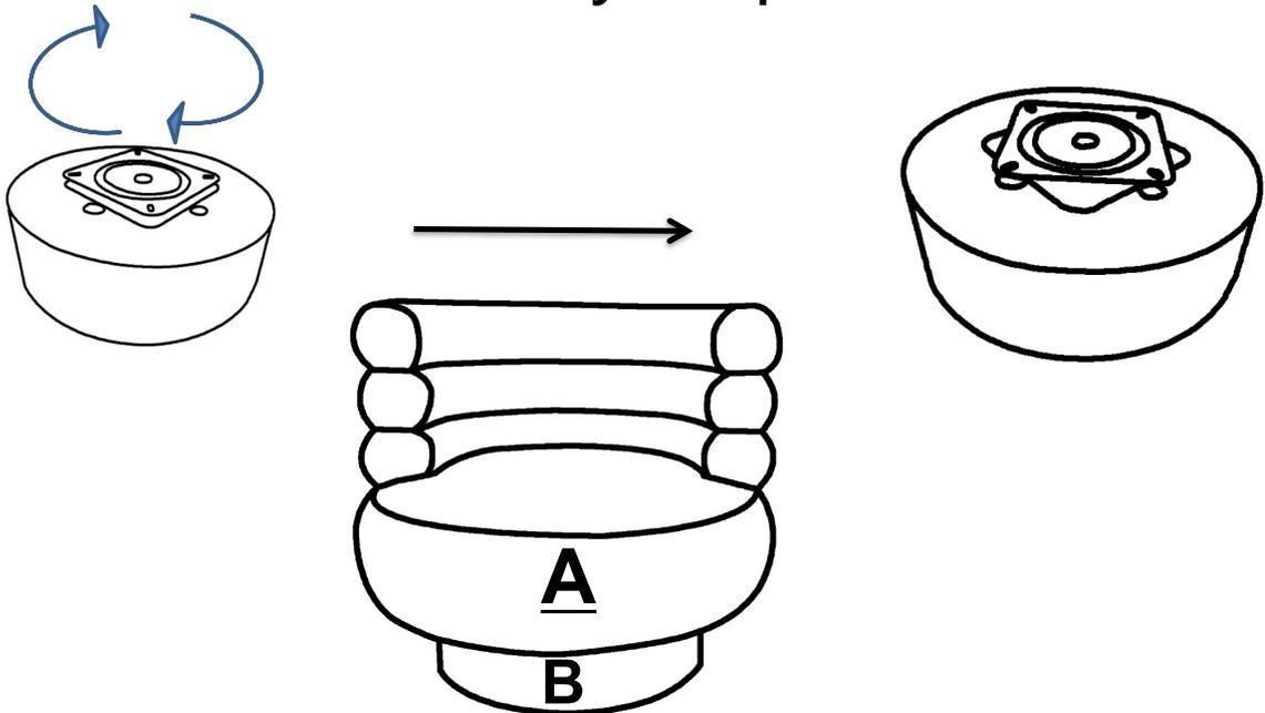
*Position the chair upside down with the base upside down on top of the chair. Align the holes in the outer plate of the swivel mechanism with the assembly holes of the chair.*
