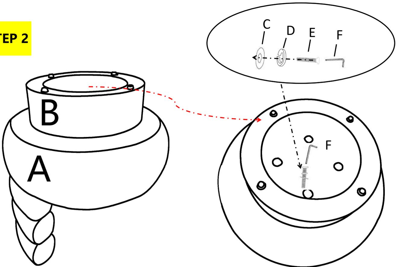
*Twist the swivel base so that the wide holes align with the holes in the outer plate of the swivel mechanism. Reaching the Allen wrench through the holes in the base, screw the swivel mechanism to the bottom of the chair.*
