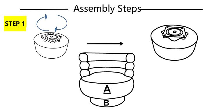
Position the chair upside down with the base upside down on top of the chair. Align the holes in the outer plate of the swivel mechanism with the assembly holes of the chair.
