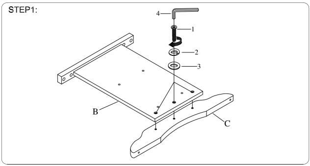
Attach leg pillar (B) to bottom leg bar (C) . Tighten by allen bolt (1), lock washer (2) and flat washer (3) with allen key (4).
