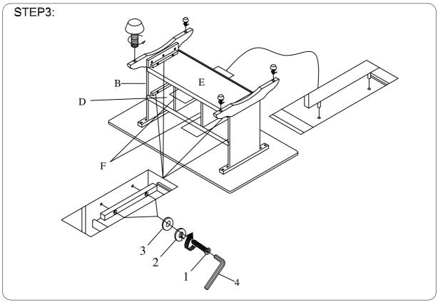
Attach center panel (F) to bottom shelf (E) and top shelf (D). Then attach bottom shelf (E) and and top shelf (D) to top leg pillar (B). Tighten by allen bolt (1), lock washer (2) and flat washer (3) with allen key (4). Tighten all bolts at this step.
