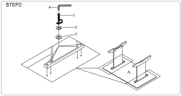
Attach leg pillar (B) to table top (A) . Tighten by allen bolt (1), lock washer (2) and flat washer (3) with allen key (4). Do not fully tighten all the bolts at this step.
