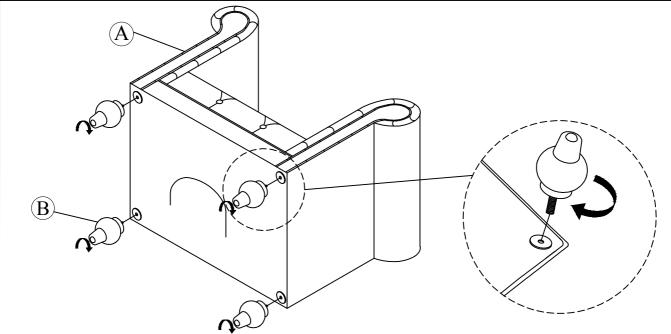
Step 2: Attach the Leg with plastic washer (B) to the Chair Body (A) as above shown.
