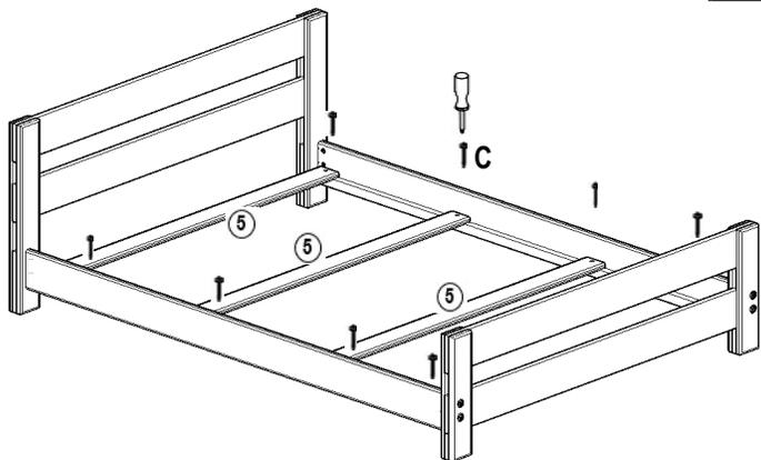
Install slats, one on each end and two equally spaced in the middle, then fasten with 1 1/4" screws
