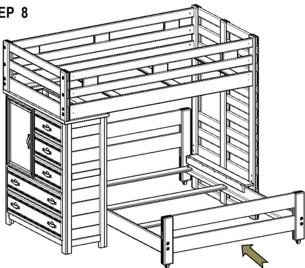
Install slats, one on each end and two equally spaced in the middle, then fasten with 1 1/4" screws
