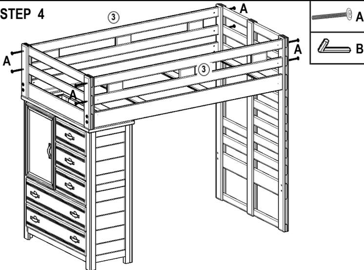
Assemble guardrails and tighten all bolts.
