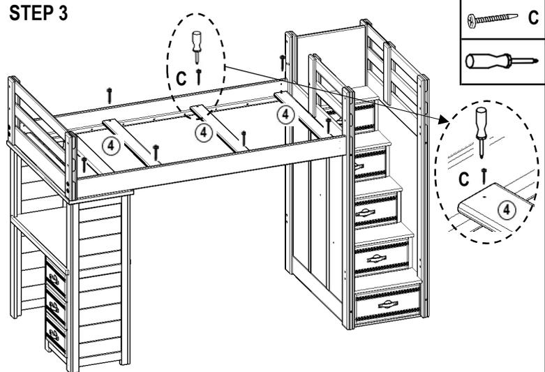
Install slats, one on each end, two equally spaced in the middle, then fasten with 1 1/4" screws.
