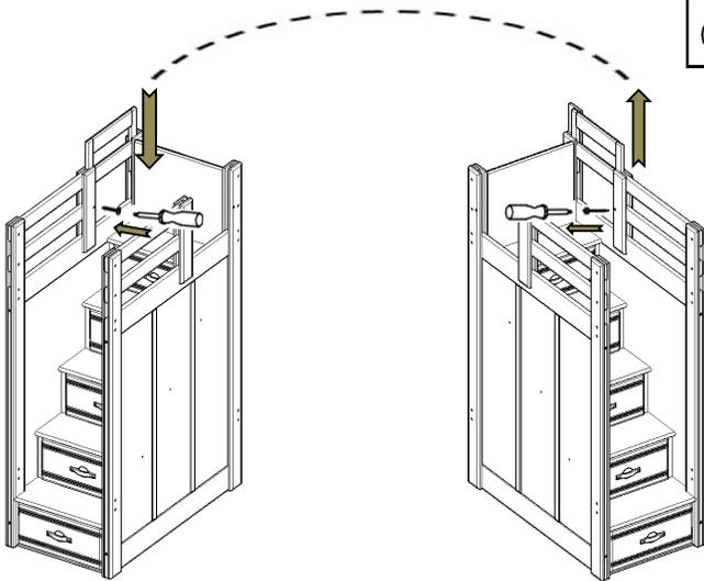
For stairs on the left, first remove the screws, then remove the panel and install it on the other side and secure with the screws.
