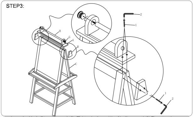
Attach wooden block (B) to side panel (C) .Tighten by Screw (1), with allen wrench(2).Then Attach top panel (A) to side panel (C) .Tighten by Screw (1), with allen wrench(2). Attach round stretcher (H) to top panel (A) .Tighten by knob (G).
