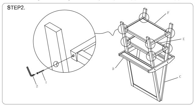
Attach middle rack (E) and bottom rack(F) to side panel (C) .Tighten by Screw (1), with allen wrench(2).
