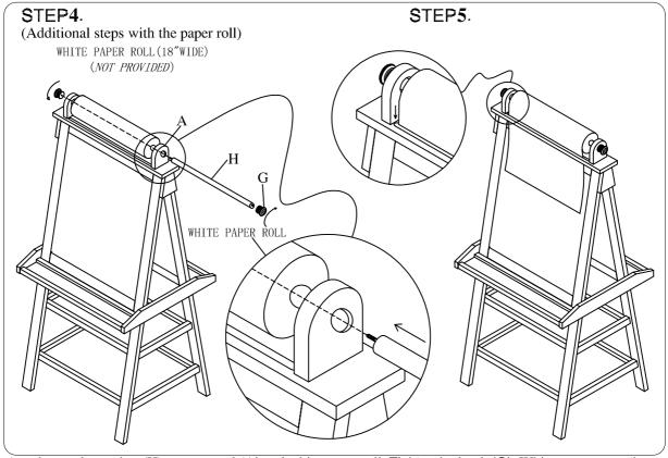
Attach round stretcher (H) to top panel (A) and white paper roll . Tighten by knob (G). White paper pass through paper slot.
