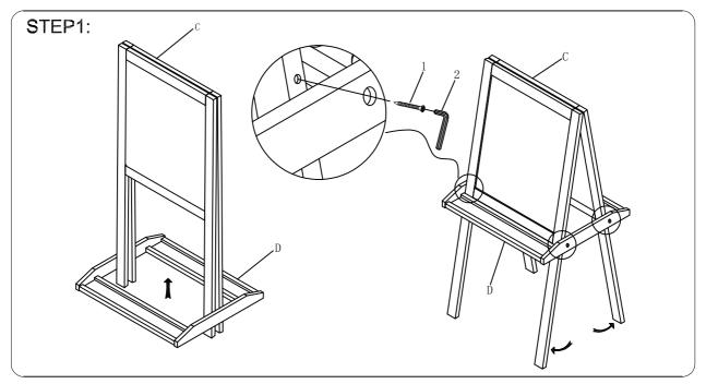
Attach side panel (C) to Top Rack (D). Tighten by Screw (1), with allen wrench(2).
