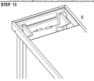
Secure each corner block with 1 1/4" screw (from desk box hardware pack) in the pre-bore hole.
