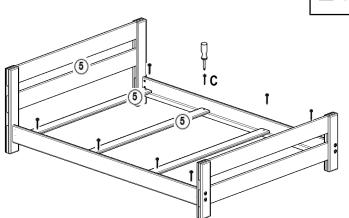
Install slats, one on each end and two equally spaced in the middle, then fasten with 1 1/4" screws
