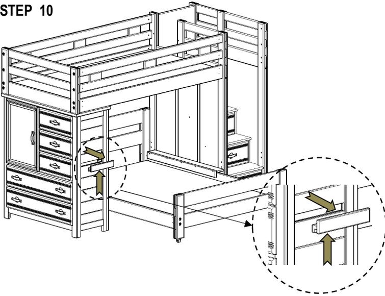
Remove center molding by lifting up then pulling out
