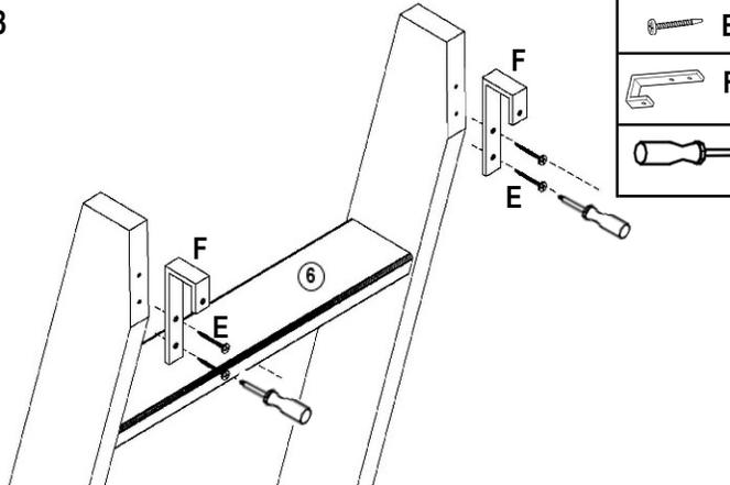
Screw ladder hooks to pre-drilled holes on top of ladder.
