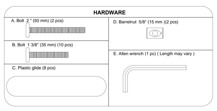
Make sure the bolts are tightly locked against the washers during assembly. (Please add an extra ½ revolution to all the bolts when using spring washer after tightening)
