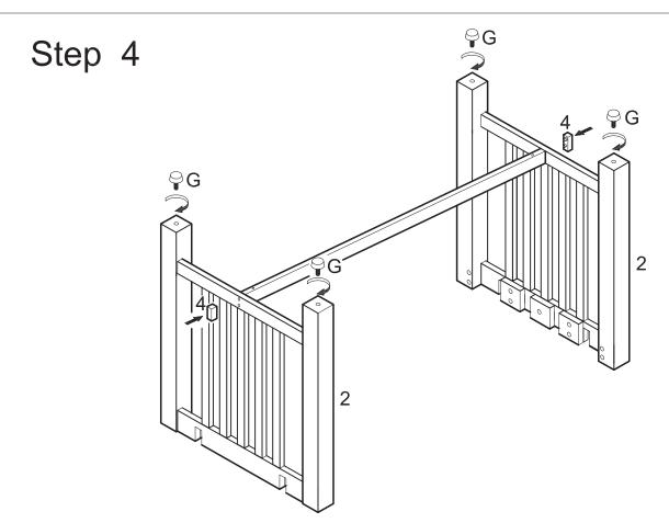
Screw feet (G) into leg pieces (2). Insert end caps (4) into leg pieces (2) using pre-inserted dowels as guides.
