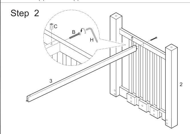
Insert nut (C) into crossbar (3). Attach crossbar (3) to leg piece (2) using bolt (B). Tighten bolt (B) with wrench(H). Bolt (B) will screw directly into nut (C).
