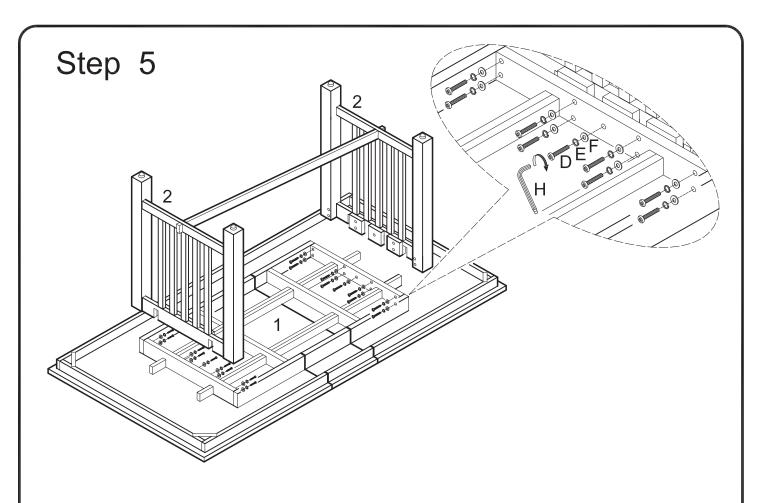
Attach leg pieces (2) to table top (1) using bolts (D), spring washers (E) and washers (F). Tighten all bolts (D) with wrench (H).
