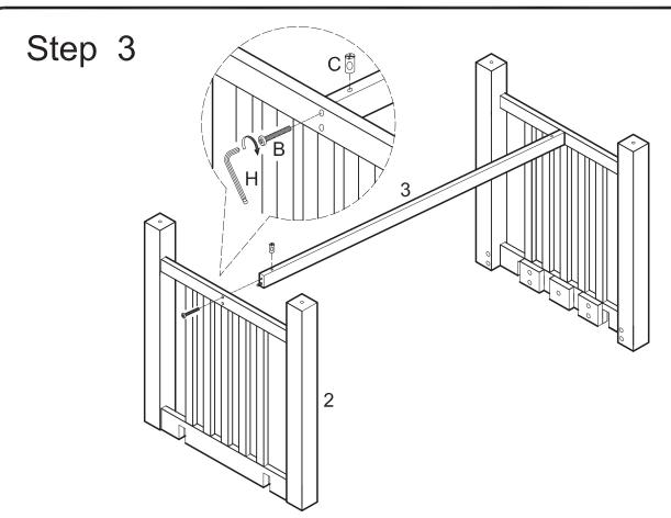
Insert nut (C) into opposite end of crossbar (3). Attach crossbar (3) to second leg piece (2) using bolt (B). Tighten bolt (B) with wrench (H). Bolt (B) will screw directly into nut (C).
