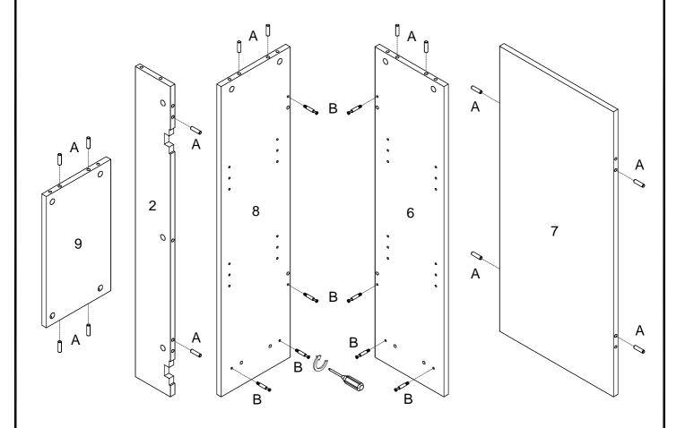
Insert wooden dowel (A) into parts (2,6,7,8,9), then using cam bolt (B) secure parts (6,8) with Philips head screwdriver as per diagram.
