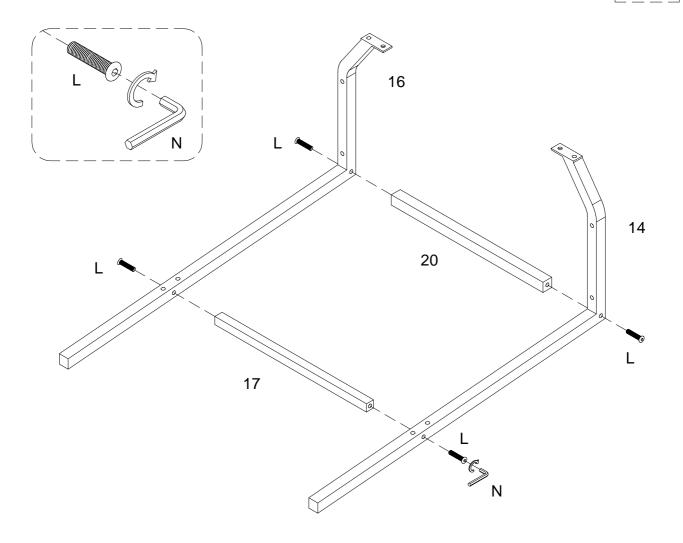
Using bolt (L) attach parts (14,16) to part (17,20) with hex key (N) as per diagram . Do not fully tighten all the bolts .
