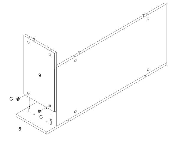
Using cam lock (C) secure part (9) into part (8) with Philips head screwdriver.
