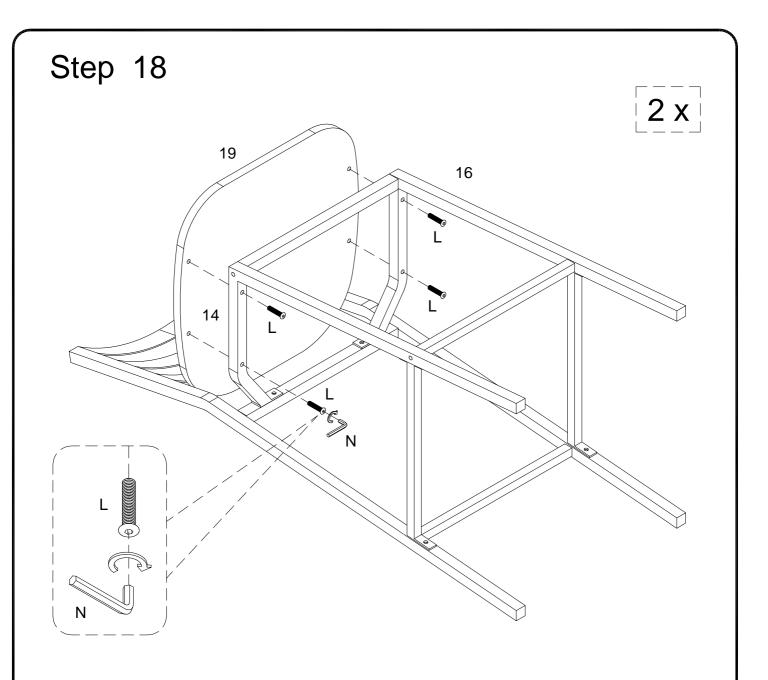
Using bolt (L) attach parts (14,16) to part (19) with hex key (N) as per diagram . And fully tighten all the bolts.
