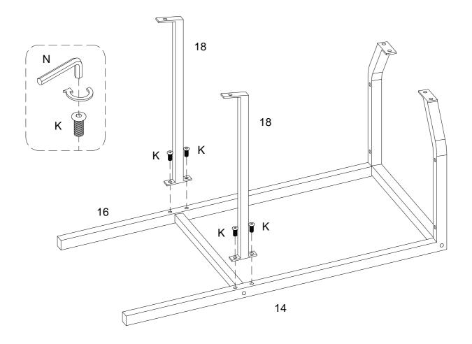
Using bolt (K) attach part (18) to parts (14,16) with hex key (N) as per diagram . Do not fully tighten all the bolts .
