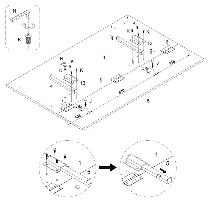
Attach rubber pad (J) on part (5) as the diagram .please keep the rubber (J) and part (4) in the same line .In this way when you pull out the leaf support (4).it could be on the rubber pad (J). Using part (13) cover part (4).then use bolt (K) secure part (13) to part (1) with hex key (N) as per diagram.
