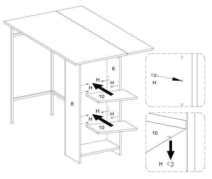
Insert shelf support pins (H) into parts (6,8) ,make sure you place the four support pins (H) in the same level so the shelf is not tilted .Then put part (10) into parts (6,8) as per diagram, tilt and rest the adjustable shelves (10) onto the shelf support pins (H).
