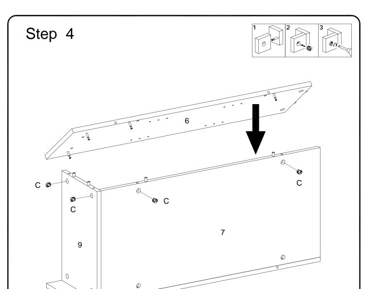
Using cam lock (C) secure part (6) into parts (7,9) with Philips head screwdriver.
