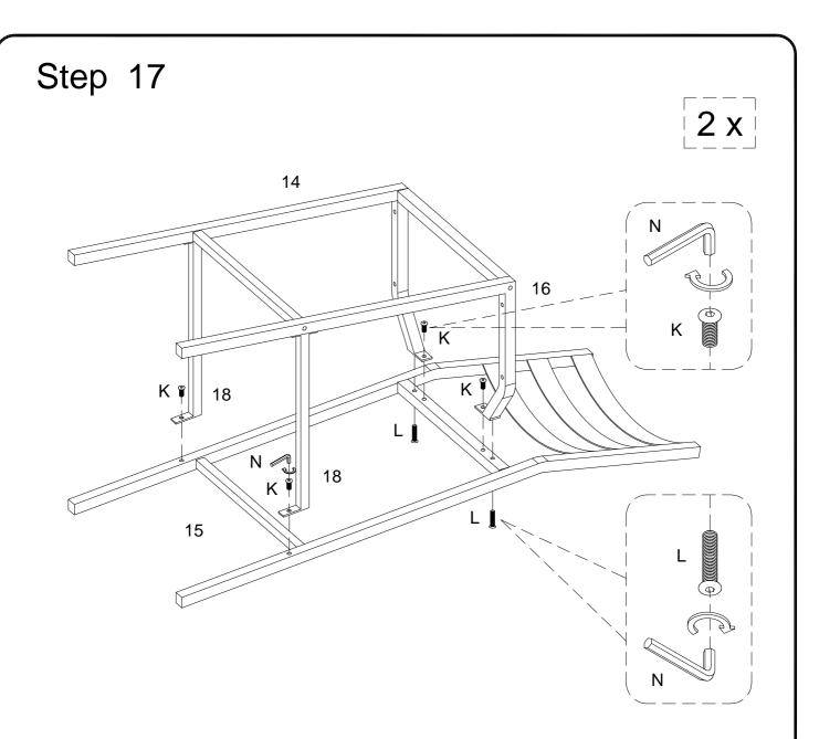
Using bolt (K) attach parts (14,16,18) to part (15) with hex key (N) as per diagram .
