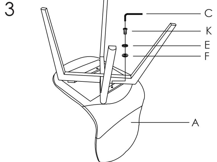
During assembly, hand tighten screws only. When the screws are in place, tighten completely.
