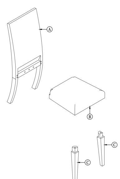
Note: Do not tighten bolt before all component assembly
