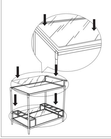
Step 6: Screw Parts F and Parts G to Parts C
