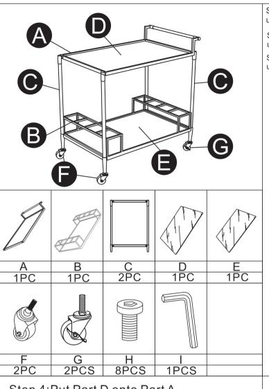
Step 1:Lay Part B with grids facing up on flat surface
