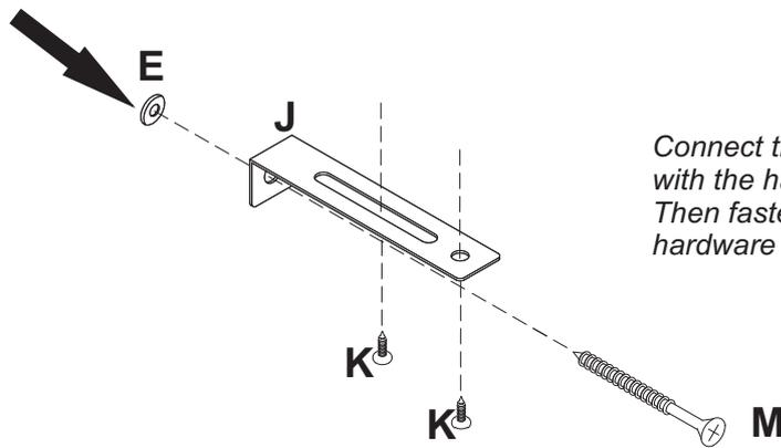
Connect the hardware (J) onto the wall with the hardware (M).
