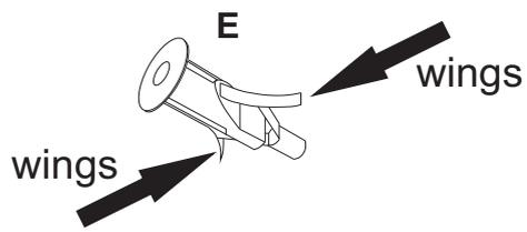
Press the hardware wings (E) to put in the hole that you drilled in the wall.
