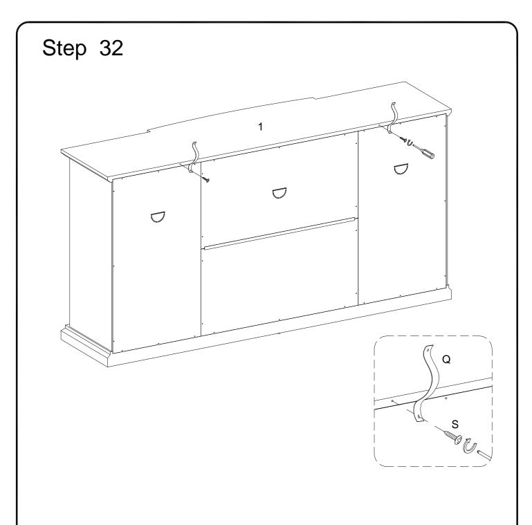
Using screw (S) attach Velcro strap (Q) to part (1) with Philips head screwdriver as per diagram.
