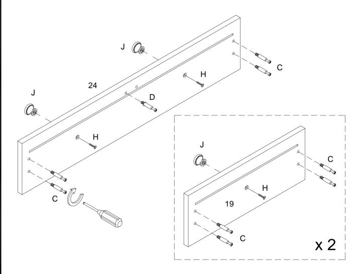
Secure cam bolt (D) to part (24) ,cam bolt (C) into parts (19,24), then using handle bolt (H) attach handle (J) to parts (19,24) with Philips head screwdriver as per diagram.
