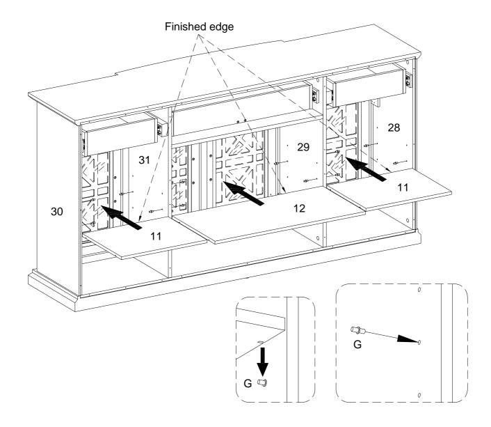
Insert shelf support pin (G) into parts (28,29,30,31) as per diagram. Make sure you place the four shelf support pins (G) in the same level. So the shelf is not titled .Put parts (11,12) into unit as per diagram. Tilt and rest the adjustable shelf(11,12) onto the shelf support pins .
