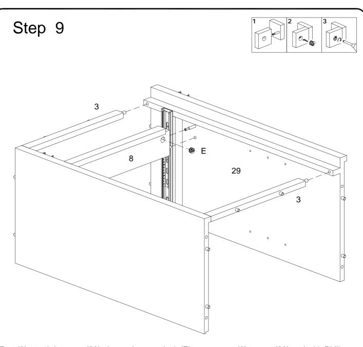
Part (3) attach into part (29) ,then using cam lock (E) secure part (8) to part (29) and with Philips head screwdriver as per diagram.
