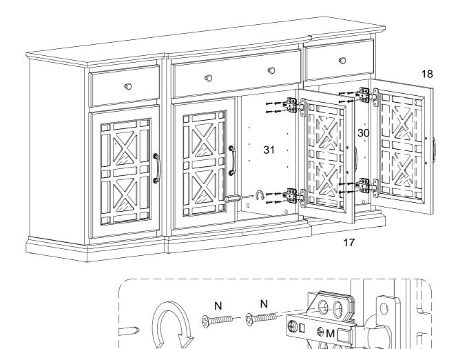
Using bolt (N) attach Europe hinge (M) into parts (30,31) with Philips head screwdriver as per diagram. Open and close the doors .If necessary adjust the screws for a good fit .
