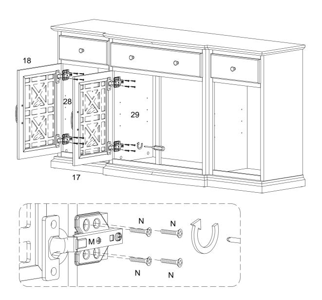
Using bolt (N) attach Europe hinge (M) into parts (28,29) with Philips head screwdriver as per diagram.
