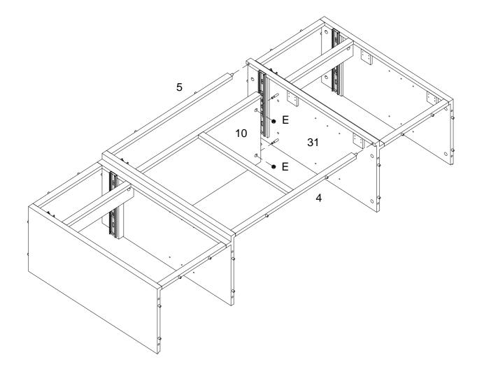
Parts (4,5) attach into part (31) ,then using cam lock (E) secure part (10) to part (31) and with Philips head screwdriver as per diagram.
