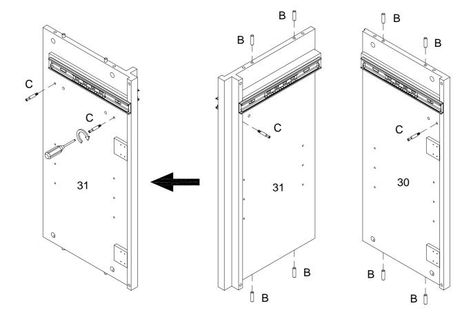
Insert wooden dowel (B) into parts (30,31), then secure cam bolt (C) into parts (30,31) with Philips head screwdriver as per diagram.
