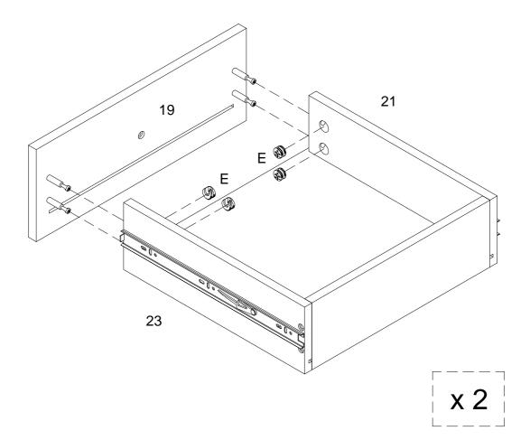
Using cam lock(E) attach part (19) to parts (21,23) with Philips head screwdriver as per diagram.
