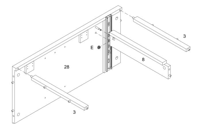
Part (3) attach into part (28) ,then using cam lock (E) secure part (8) to part (28) and with Philips head screwdriver as per diagram.
