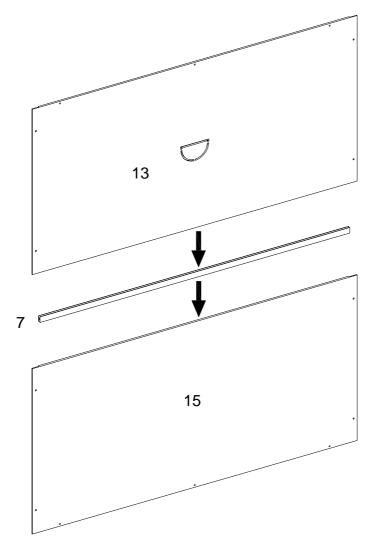
Attach parts (7,13,15) as per diagram.
