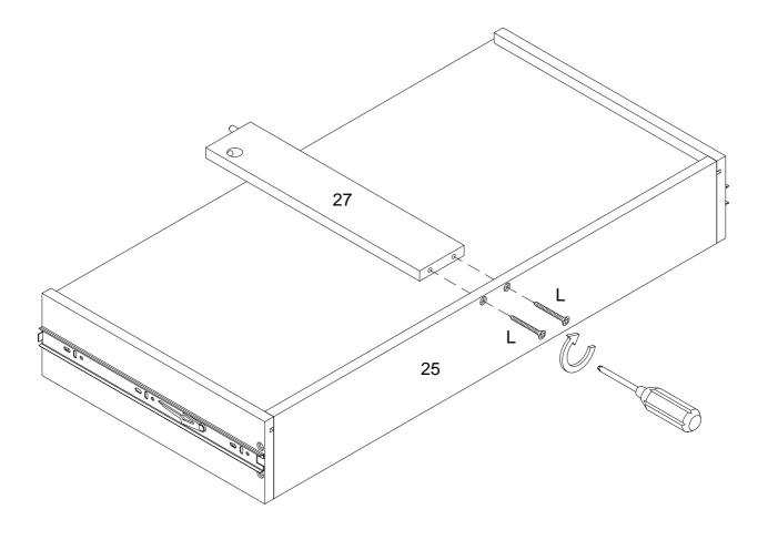
Using Flat head screw (L) attach part (25) into part (27) with Philips head screwdriver as per diagram.
