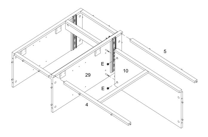
Parts (4,5) attach into part (29) ,then using cam lock (E) secure part (10) to part (29) and with Philips head screwdriver as per diagram.
