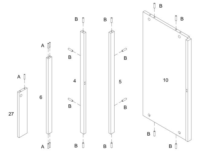
Insert wooden dowel (A) into parts (6,27), wooden dowel (B) into parts (4,5,10) as per diagram.
