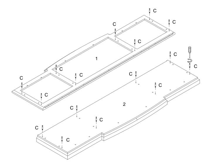
Secure cam bolt (C) into parts (1,2) with Philips head screwdriver as per diagram.
