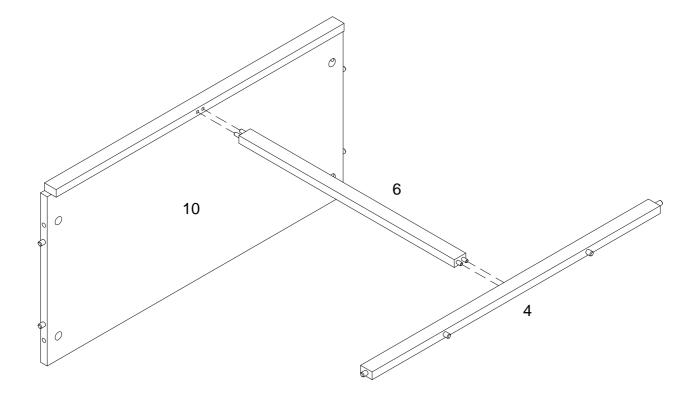
Part (6) insert to parts (4,10) as per diagram.
