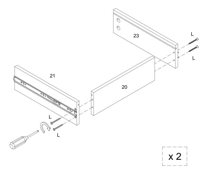
Using Flat head screw (L) attach parts (21,23) to part (20) with Philips head screwdriver as per diagram.
