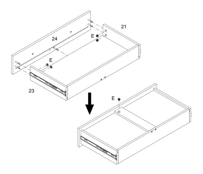
Using cam lock(E) attach part (24) to parts (21,23) with Philips head screwdriver as per diagram.
