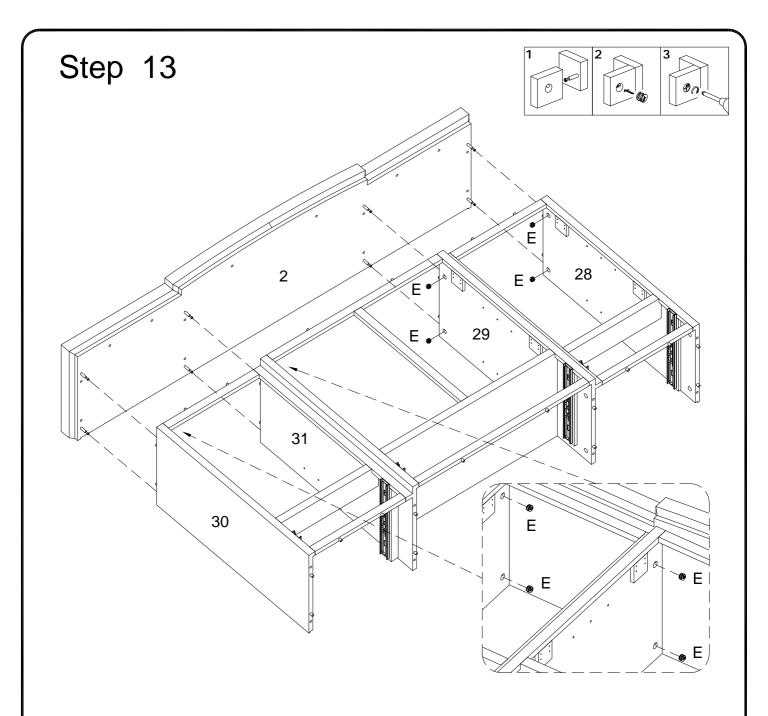
Using cam lock (E) attach part (2) to parts (28,29,30,31) with Philips head screwdriver as per diagram.
