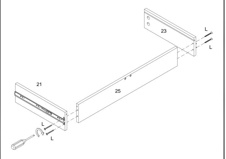
Using Flat head screw (L) attach parts (21,23) to part (25) with Philips head screwdriver as per diagram.
