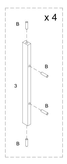
Insert wooden dowel (B) into parts (3,8,9) as per diagram.
