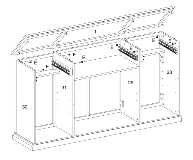
Using cam lock (E) attach part (1) to parts (28,29,30,31) with Philips head screwdriver as per diagram.
