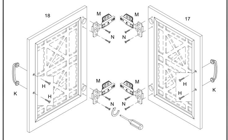
Using bolt (N) attach Europe hinge (M) ,Handle bolt (H) attach handle (K) into parts (17,18)with Philips head screwdriver as per diagram.
