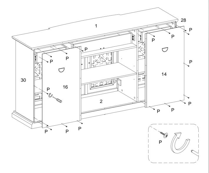
using flat head screw (P) attach part (14) to parts(1,2,28),part(16) to parts(1,2,30) with Philips head screwdriver as per diagram.
