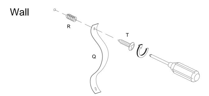
Using screw (T) attach plastic strap (Q) into nut (R) to wall with Philips head screwdriver as per diagram.
