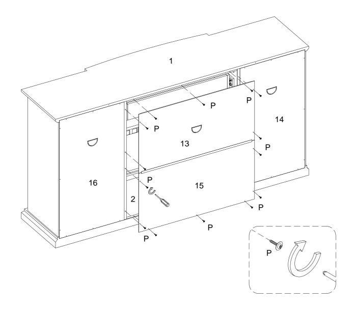
Using Flat head screw (P) attach parts (13,15) into parts (1,2,29,31) with Philips head screwdriver as per diagram.
