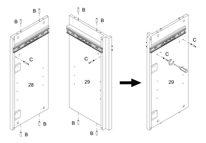
Insert wooden dowel (B) into parts (28,29), then secure cam bolt (C) into parts (28,29) with Philips head screwdriver as per diagram.
