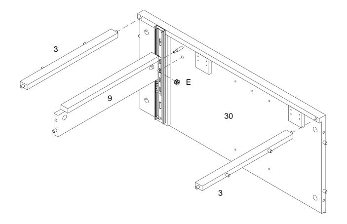
Part (3) attach into part (30) ,then using cam lock (E) secure part (9) to part (30) and with Philips head screwdriver as per diagram.
