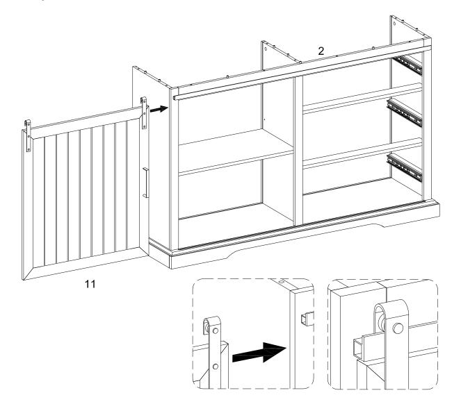
Pick up the door (11), and fit the pulley over the slider rails on part (2) as per diagram.
