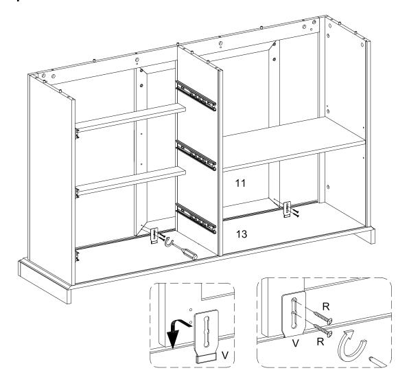
Place the plate (V) into the slider rail on the bottom panel, using screw (R) attach plate (V) to part (11) with Philips head screwdriver as per diagram.
