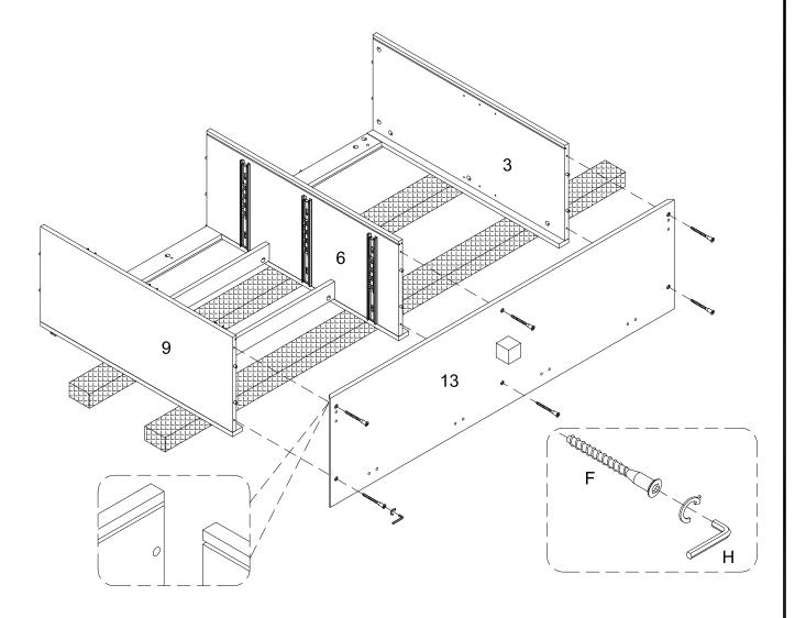
Using screw (F) attach part (13) to parts (3,6,9) with hex key (H) as per diagram.
