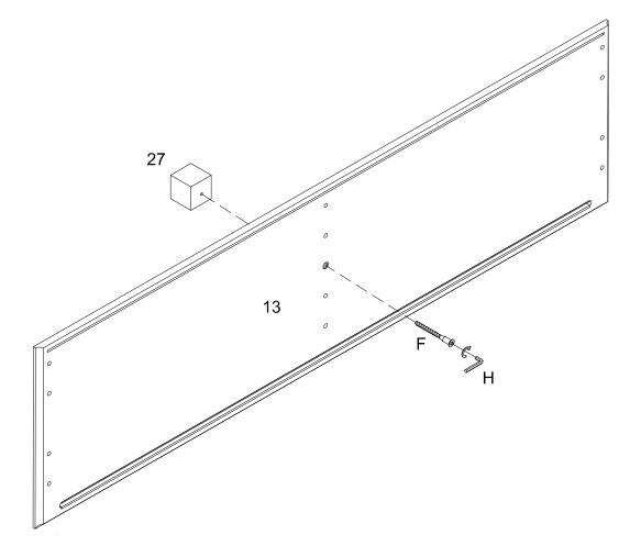
Using screw (F) attach part (27) to part (13) with Hex Key (H) as per diagram.
