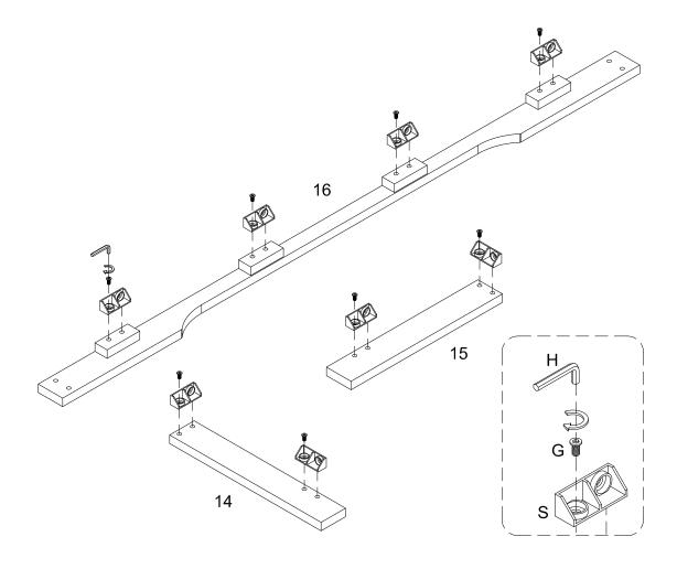
Using bolt (G) secure plastic wedge (S) into parts (14,15,16) with Hex key (H) as per diagram.
