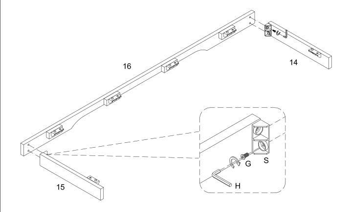
Using bolt (G) secure plastic wedge (S) into part(16) with Hex key (H) as per diagram.
