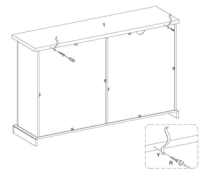
Using screw (R) attach Velcro strap (Y) into part (1) with Philips head screwdriver as per diagram.
