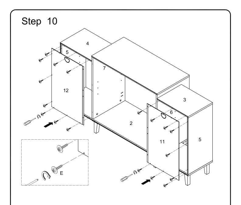
Using screw (E) secure part(11) to parts (2,3,5);part (12)to parts (2,4,5) with a Philips screwdriver as per diagram.
