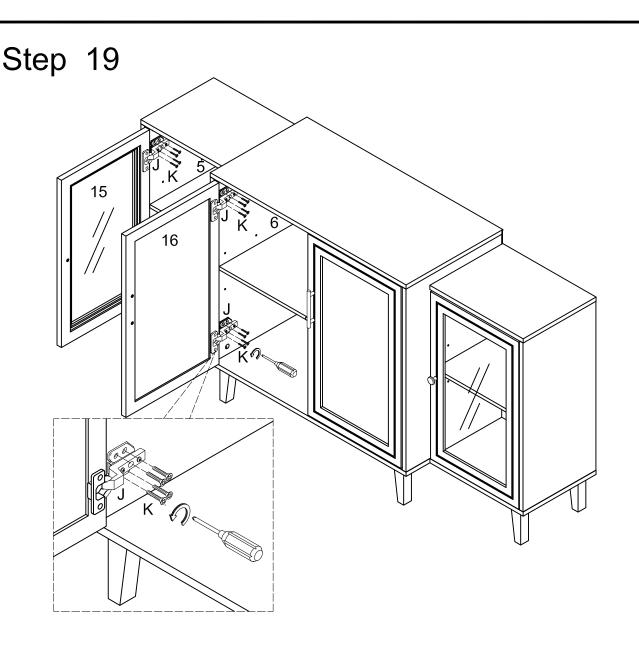
Using screw (K)secure Europe hinge (J) to parts (5,6)with Philips screwdriver as per diagram. After assembled the four doors . please close and open the doors to make sure they are align and shut correctly ,if necessary adjust the screw (K) for a good fit .
