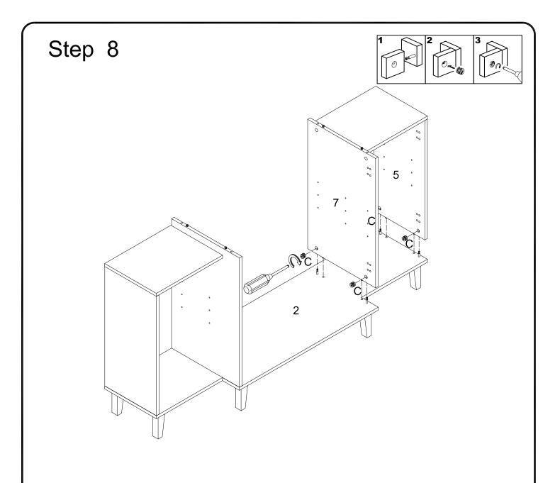
Using cam locks (C) attach parts(5,7) to part (2) with a Philips screwdriver as per diagram.
