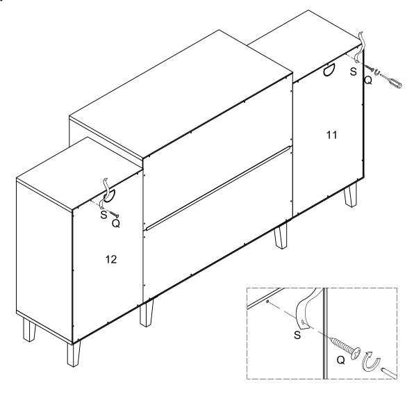
Using screw (Q) secure the part (S)to back panels (11,12) a Philips screwdriver as per diagram.
