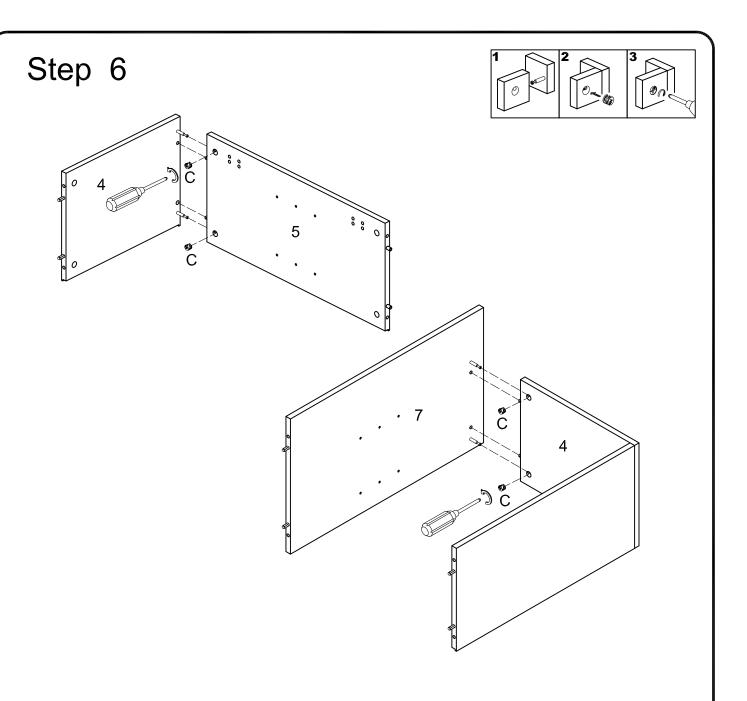
Using cam locks(C) attach part (4) to part(5) and then using cam locks(C)attach the other side of part (4) to part (7)with a Philips screwdriver as per diagram.
