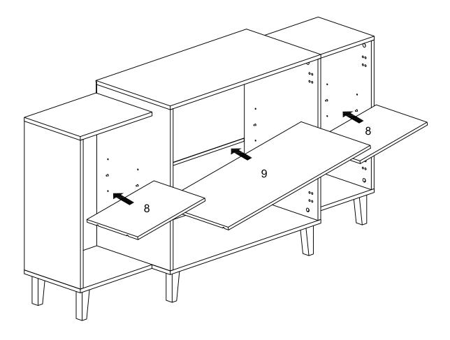
Make sure you place the four shelf pins in the same level so the shelf is not tilted . Tilt and rest the adjustable shelves (8,9) onto the shelf support pin (D)as per diagram .
