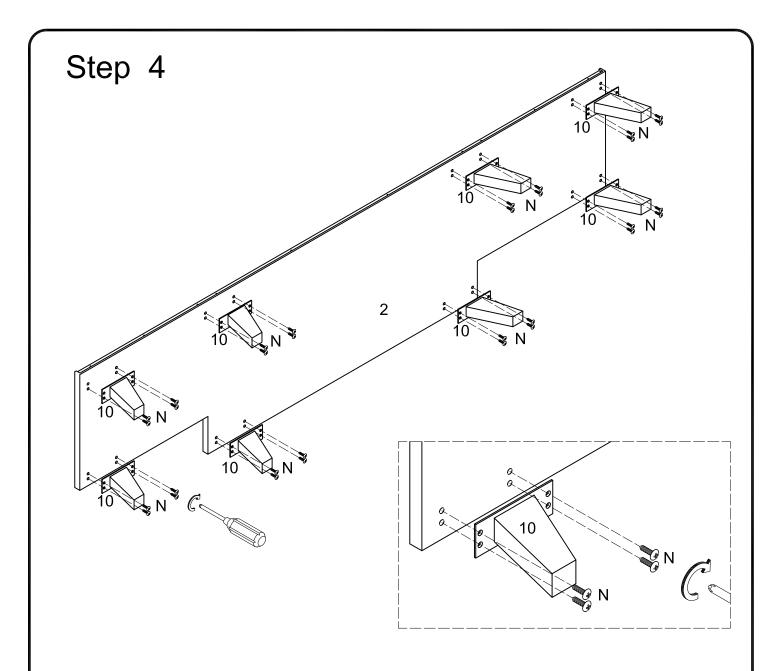
Using screw (N) attach the leg (10) to bottom panel (2) with a Philips screwdriver as per diagram. Please kindly noted the legs placed the same direction as the AI shows .
