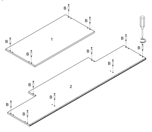
Securely screw the cam bolts (B) on parts (1 and 2) with a Philips screwdriver as per diagram .
