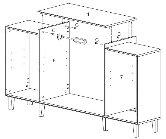
Align and attach part(1) with parts(6,7) with cam locks (C) with a Philips screwdriver as per diagram.
