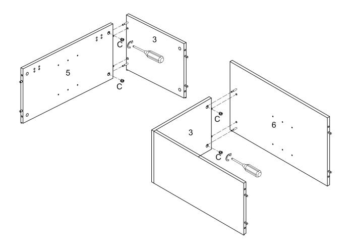
Using cam locks(C) attach part (3) to part(5) and then using cam locks(C)attach the other side of part (3) to part (6)with a Philips screwdriver as per diagram.
