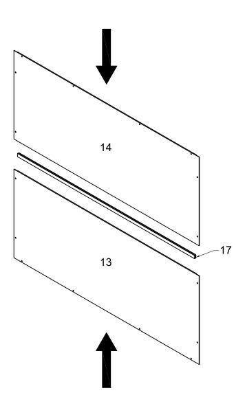
Attach parts(13,14) with part (17) as per diagram
