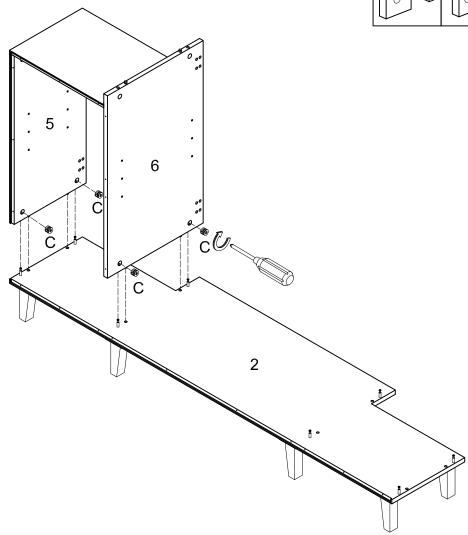
Using cam locks (C) attach parts(5,6) to part (2) with a Philips screwdriver as per diagram.
