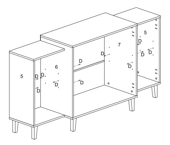
Insert shelf support pin (D) into parts (5,6,7) as per diagram .
