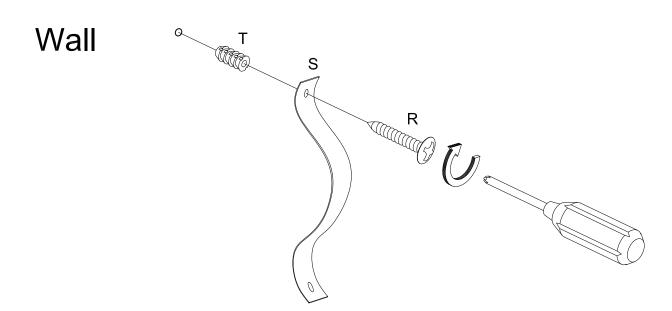
Insert the plastic nut (T) into the wall and using screw (R) fix the other side of strap (S) with nut (T) in the wall .The unit is now ready for use .
