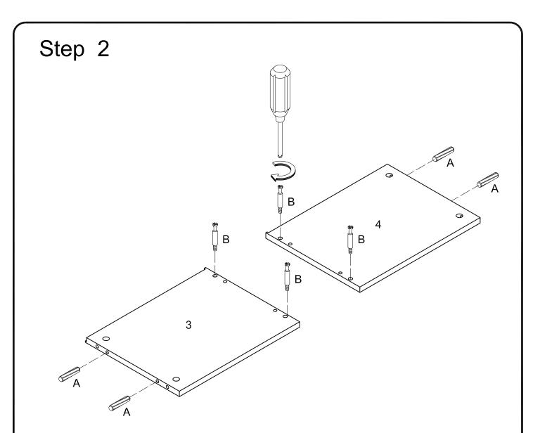
Insert wooden dowels into parts (3,4). Securely screw the cam bolts (B) on parts (3 and 4) with a Philips screwdriver as per diagram.
