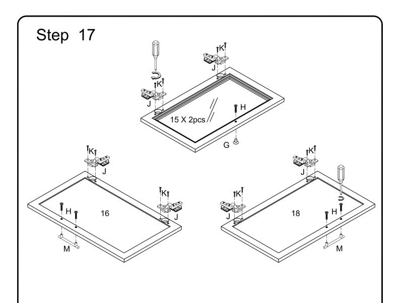
Using handle bolt (H) secure handle (G) to part(15); handle (M) to parts (16,18), then using screw (K) secure Europe hinge (J) to parts (15,16,18) with a Philips screwdriver as per diagram.
