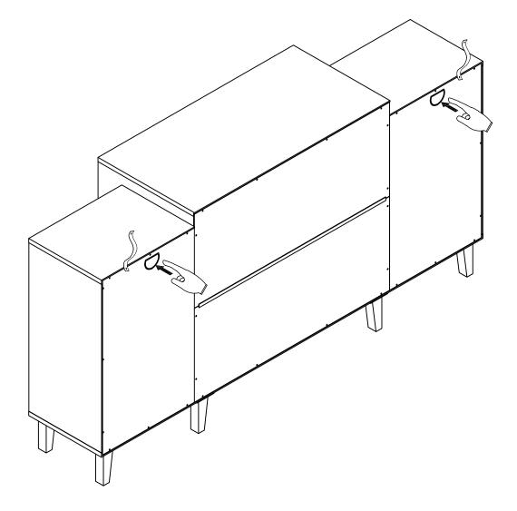
Take out the wooden panel of the faux cable holes if necessary .
