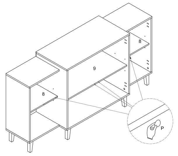
Stick the rubber pad on front of the adjustable shelves (8,9) as per diagram .
