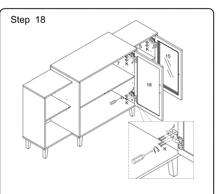
Using screw (K) secure Europe hinge (J) to parts (5,7) with a Philips screwdriver as per diagram.
