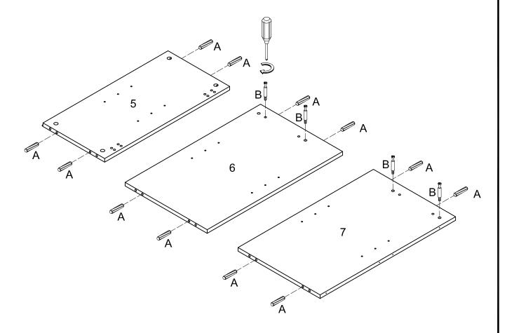
Insert wooden dowels into parts (5,6,7). Securely screw the cam bolts (B) on parts (6 and 7) with a Philips screwdriver as per diagram.
