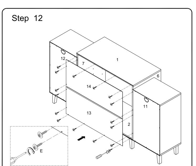
Using screw (E) secure part (13) to parts (2,6,7,11,12),part (14) to parts(1,6,7,11,12) with Philips screwdriver as per diagram.
