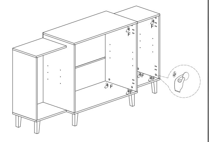
Using sticker (F) cover the cam lock holes as per diagram.
