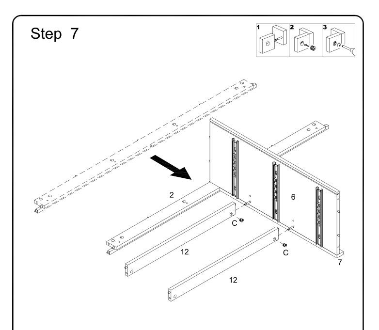
Attach part (2) to part (7),then using Cam lock(C) secure part (12) to part (6) with Philips head screwdriver as per diagram.
