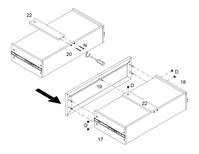
Using screw (N) attach part (20) to part (22) ,then using cam lock (D) secure part (19) to parts(17,18,22) with Philips head screwdriver as per diagram.
