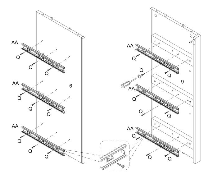
Using screw (Q) secure drawer slider (AA) to parts (6,9) with Philips head screwdriver as per diagram.
