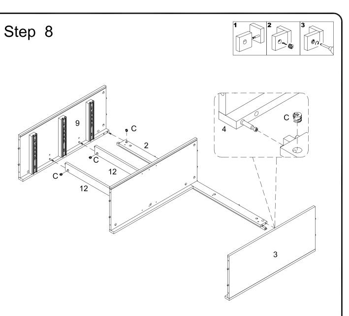
Using Cam lock(C) secure parts (2,12) to part (9) ,parts (3,2) to part (3) with Philips head screwdriver as per diagram.
