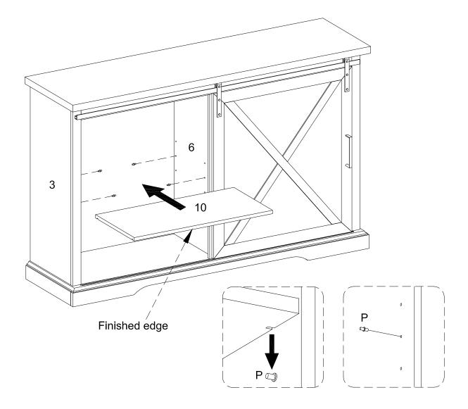
Insert shelf support pin (P) into parts (3,6) as per diagram. Make sure you place the shelf support pins (P) in the same level. So the shelf is not titled .Put part (10) into unit as per diagram. Tilt and rest the adjustable shelf(10) onto the shelf support pins .
