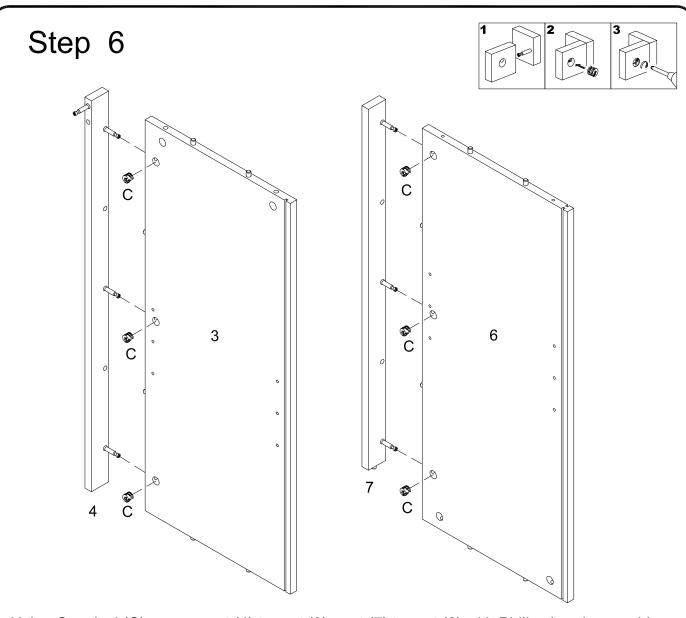
Using Cam lock(C) secure part (4) to part (3) ,part (7) to part (6) with Philips head screwdriver as per diagram.
