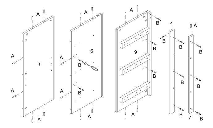
Insert wooden dowel (A) into parts (3,6,7,9), then secure cam bolt (B) into parts (4,6,7,9) with Philips head screwdriver as per diagram.
