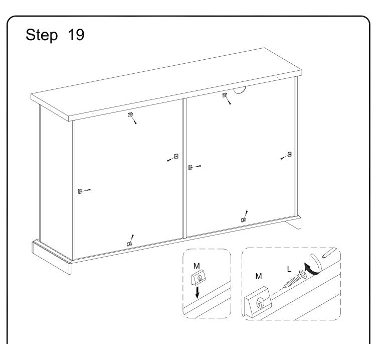
Using screw (L) secure plastic wedge (M) with Philips head screwdriver as per diagram.
