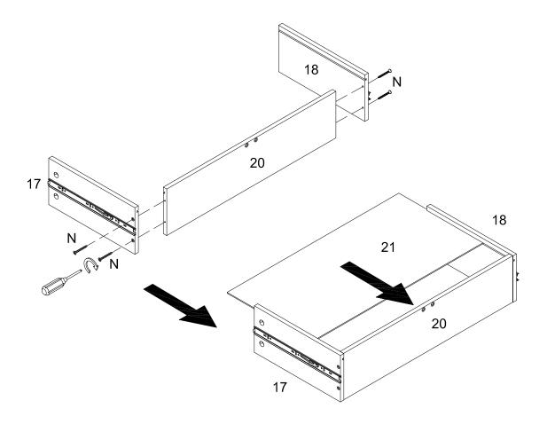
Using screw (N) attach parts (17,18) to part (20) with Philips head screwdriver ,then put part (21) as per diagram.
