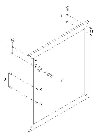
Using bolt (U) secure Pulley (T) into part (11) ,and using bolt (K) secure Handle (J) into parts (11) with Philips head screwdriver as per diagram.
