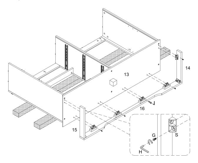
Using bolt (G) secure plastic wedge (S) into part (13) with Hex key (H)as per diagram.
