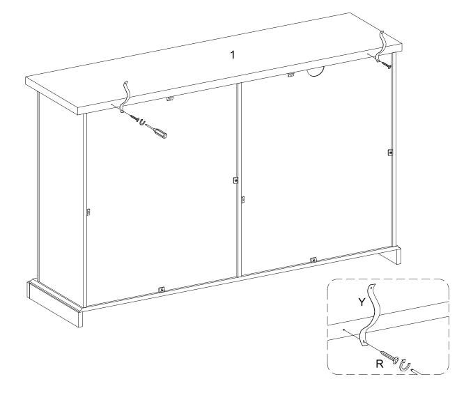
Using screw (R) attach Velcro strap (Y) into part (1) with Philips head screwdriver as per diagram.
