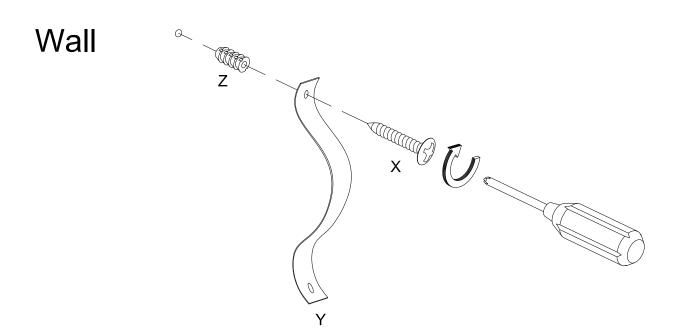
Using screw (X) attach Velcro strap (Y) into Nut (Z) to wall with Philips head screwdriver as per diagram.
