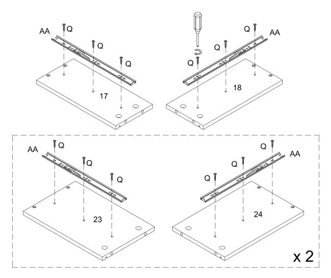
Using screw (Q) secure drawer slider (AA) to parts (17,18,23,24) with Philips head screwdriver as per diagram.
