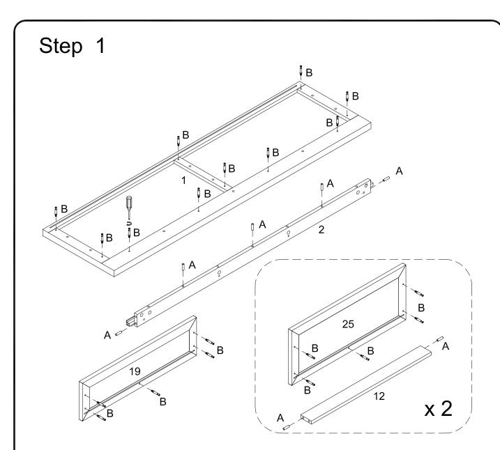
Insert wooden dowel (A) into parts (2,12) ,then secure cam bolt (B) into parts (1,19,25) with Philips head screwdriver as per diagram.
