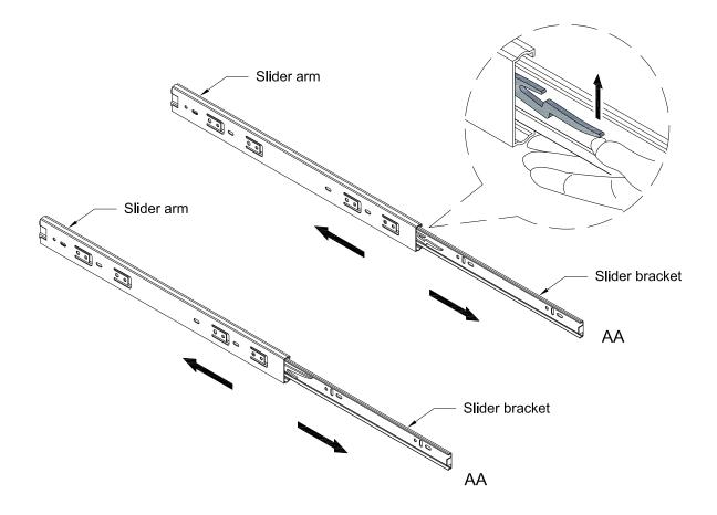
Pick up the slider (AA) and separate the slider arm and slider bracket for the following steps. Extend the Slide .Runner all the way forward, press the plastic release lever of the slider bracket and pull out the Slider bracket complete.
