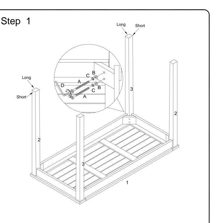
Using bolts (A) with Lock washer (C) and Flat washer (B) attach part (1) to parts (2,3) with hex key (D) as per diagram.
