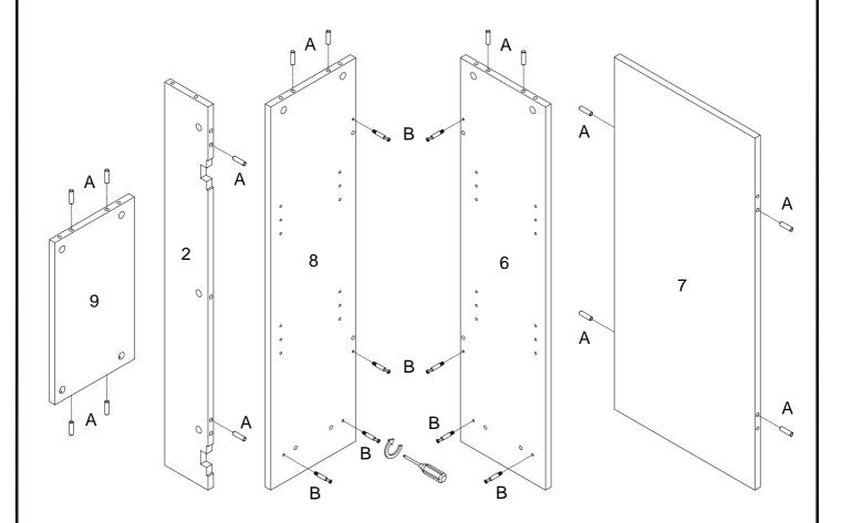
Insert wooden dowel (A) into parts (2,6,7,8,9), then using cam bolt (B) secure parts (6,8) with Philips head screwdriver as per diagram.
