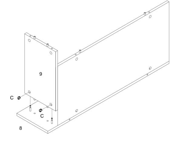
Using cam lock (C) secure part (9) into part (8) with Philips head screwdriver.
