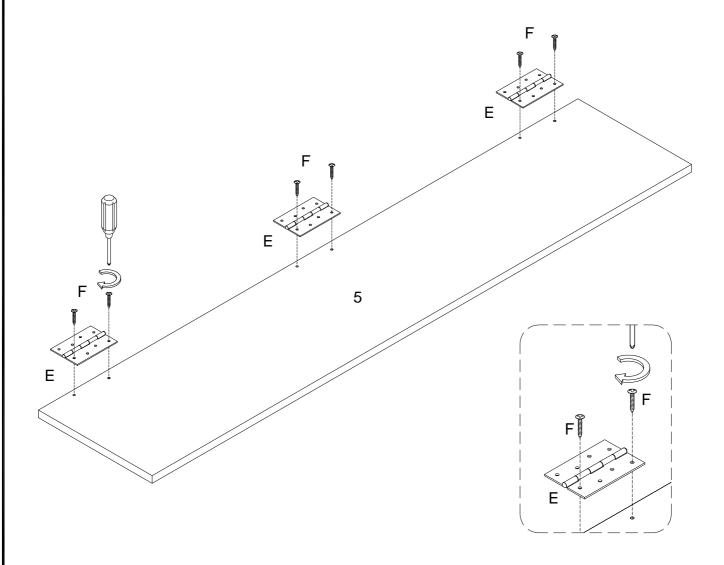
Using screw (F) attach hinge (E) into part (5) with Philips head screwdriver as per diagram .
