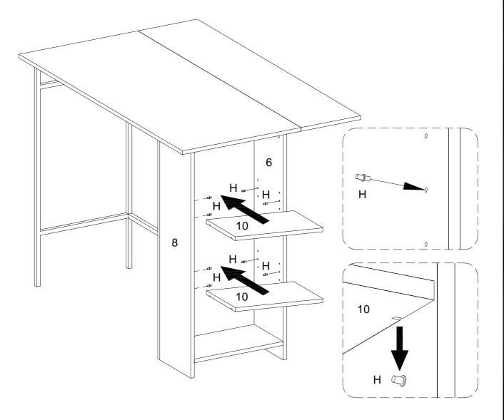
Insert shelf support pins (H) into parts (6,8), make sure you place the four support pins (H) in the same level so the shelf is not tilted .Then put part (10) into parts (6,8) as per diagram, tilt and rest the adjustable shelves (10) onto the shelf support pins (H).
