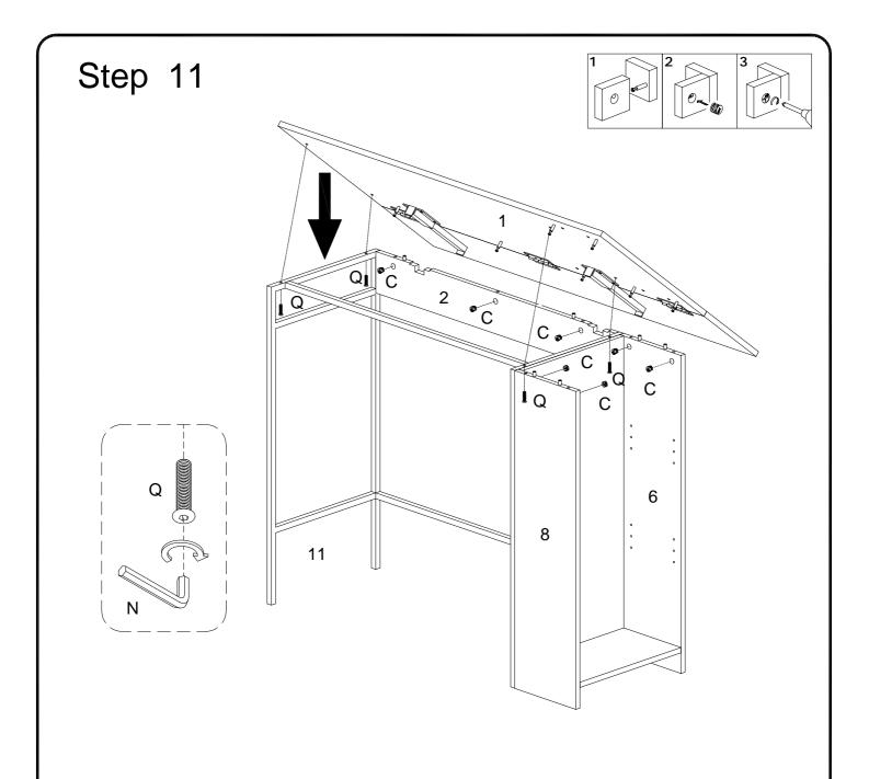
Using bolt (Q) secure part (1) into part (11,12) with hex key (N), then using cam lock (C) secure part (1) into parts (2,6,8) with Philips head screwdriver as per diagram.
