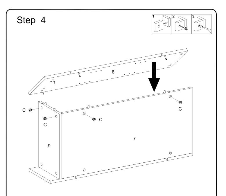
Using cam lock (C) secure part (6) into parts (7,9) with Philips head screwdriver.
