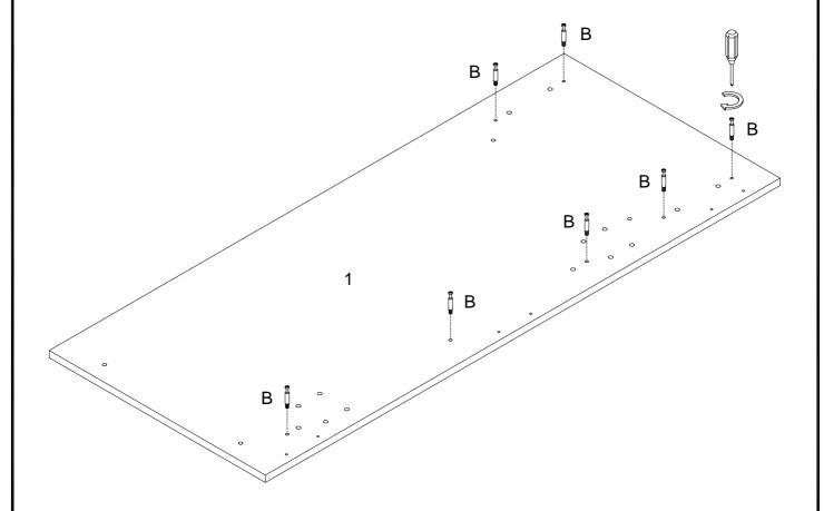
Using cam bolt (B) secure part (1) with Philips head screwdriver.
