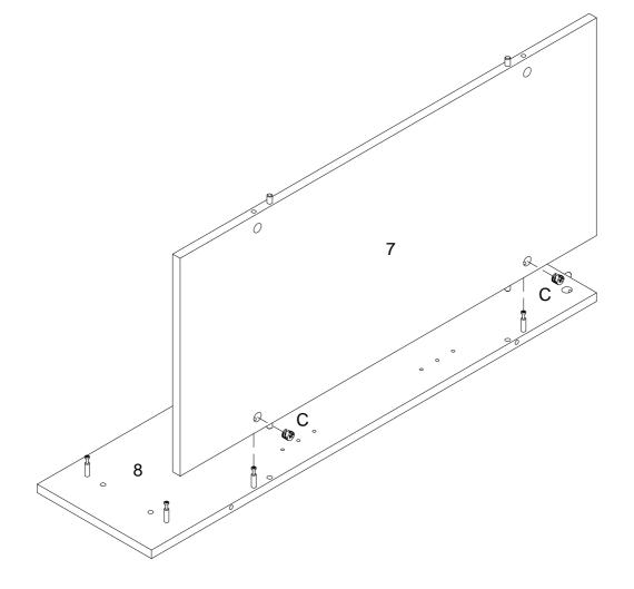
Using cam lock (C) secure part (7) into part (8) with Philips head screwdriver.
