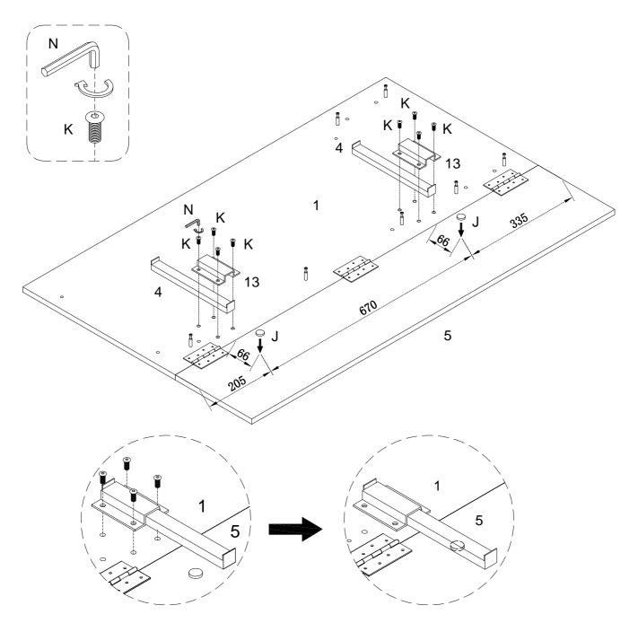
Attach rubber pad (J) on part (5) as the diagram .please keep the rubber (J) and part (4) in the same line .In this way when you pull out the leaf support (4).it could be on the rubber pad (J). Using part (13) cover part (4).then use bolt (K) secure part (13) to part (1) with hex key (N) as per diagram.
