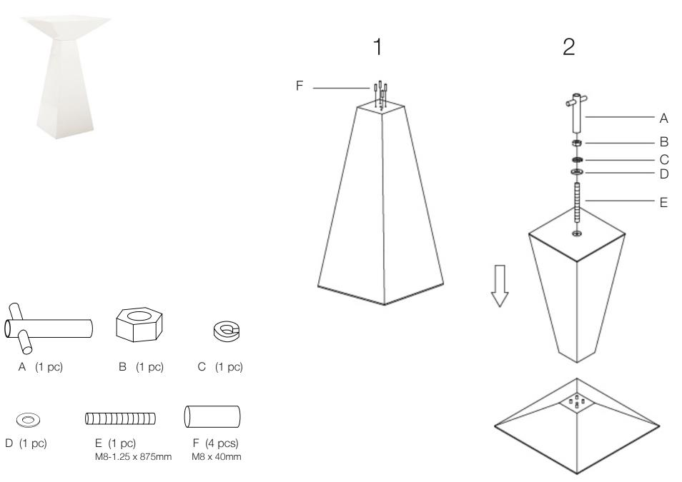
During assembly, hand tighten screw only. When the screw is in place, tighten completely.
