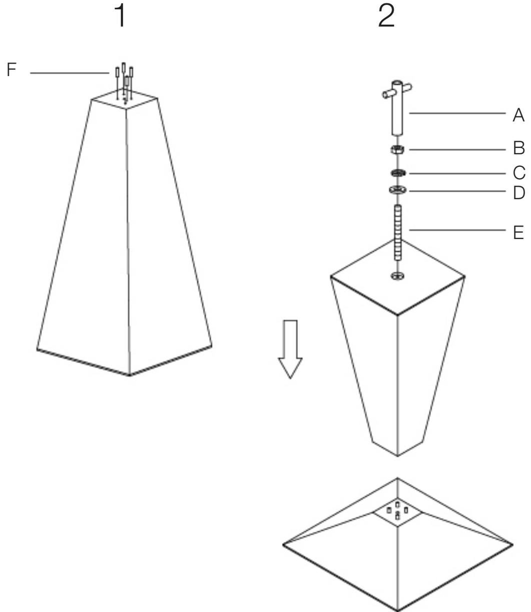
During assembly, hand tighten screw only. When the screw is in place, tighten completely.
