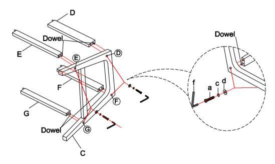
Step 2. Repeat the step 1 to attach the left leg (B) to the rails and stretchers (D,E,F,G) using bolts (a), lock washers (c) and flat washers (d). Securely tighten all bolts by Allen wrench (f), but do not over tighten the bolts.
