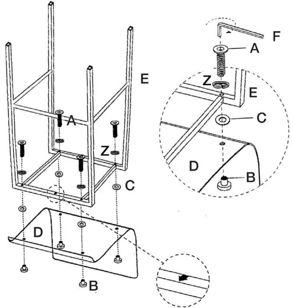
During assembly, hand tighten screws only. When the screws are in place, tighten completely.
