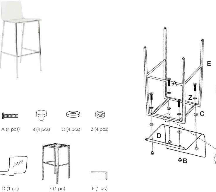
During assembly, hand tighten screws only. When the screws are in place, tighten completely.
