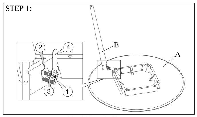
Attach the table leg to the table frame. Note: Do not tighten all screws & bolts until the table is fully assembly.
