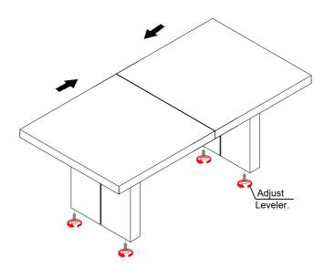
Close Table Top,Close locks, Apply firm pressure to align Leveler.
