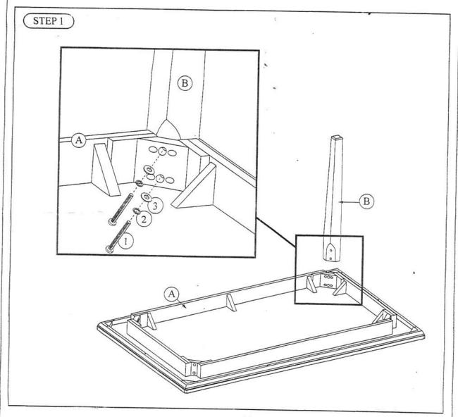
Attach the Legs (B) to the Top (A) using 2 Allen Bolts (1), 2 Spring Washers (2), and 2 Flat Washers (3) from the inside.
